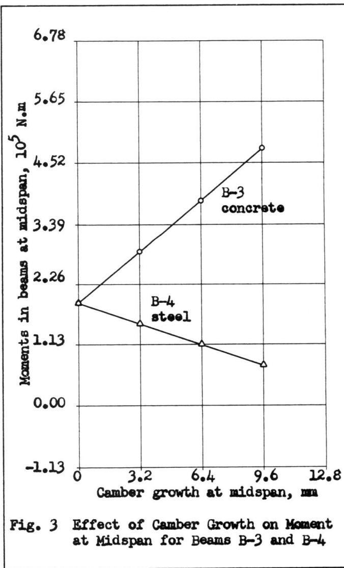
Fig. 3 Effect of Camber Growth on Moment at Midspan for Beams B-3 and B-4
