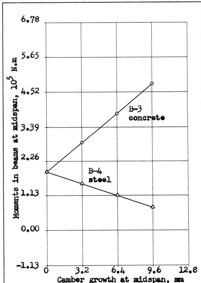
Fig. 3 Effect of Camber Growth on Moment at Midspan for Beams B-3 and B-4
