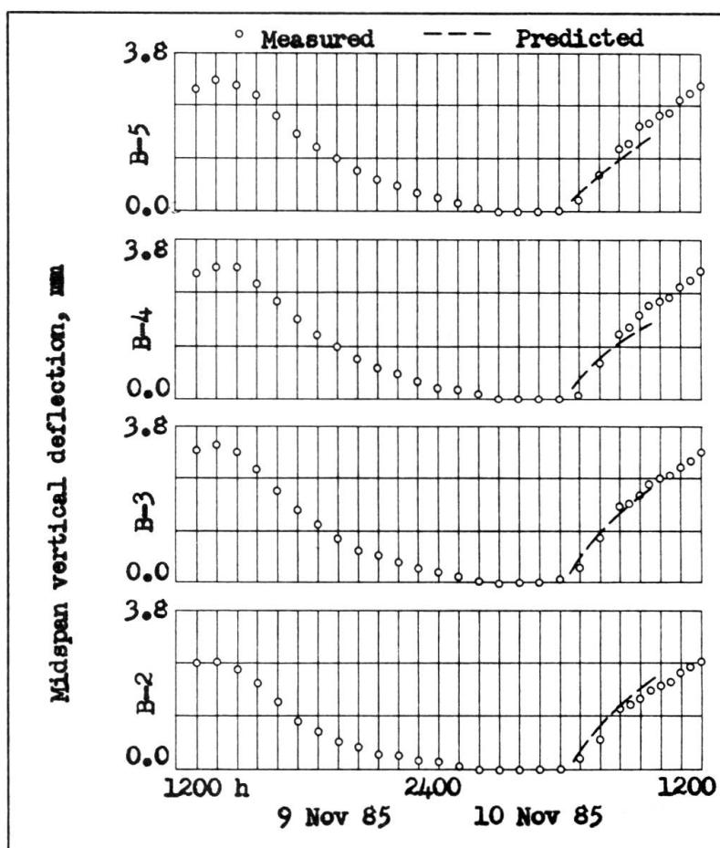
Fig. 4 Predicted vs. Measured Thermally Induced Deflections as a Function of Time of Day
