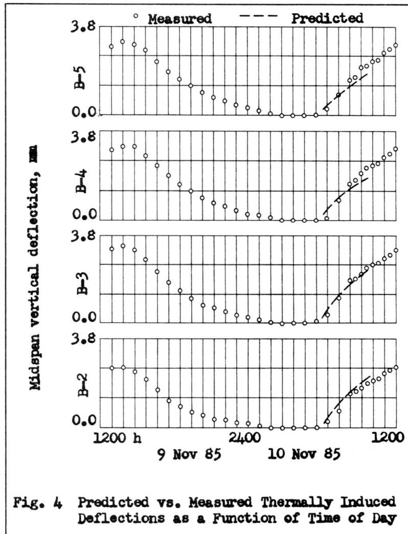
Fig. 4 Predicted vs. Measured Thermally Induced Deflections as a Function of Time of Day
