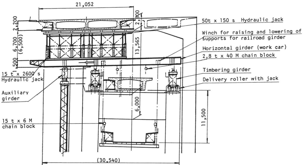
Fig. 10 Erection by Movable Staging (Cross Section)
