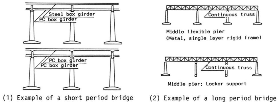
Fig. 17 Comparison of Bridge Pier for Bannosu Viaduct
