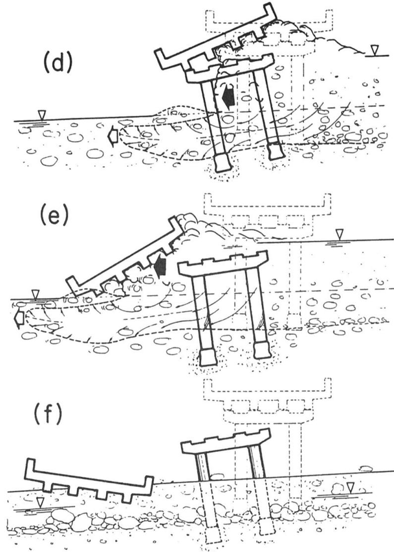
FIG. 4 SCHEMATICAL VIEW OF PROPOSED FAILURE MECHANISM
