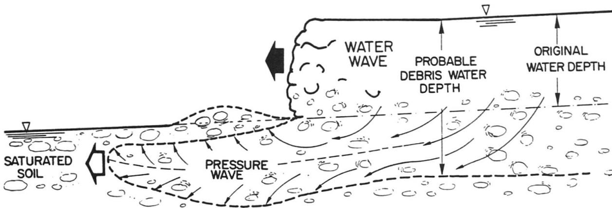
FIG. 3 SCHEMATIC VIEW OF A FLASH FLOOD WAVE.
