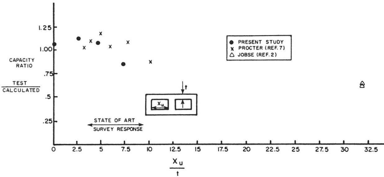
Fig. 7 Effect of wall thickness on pier capacity
