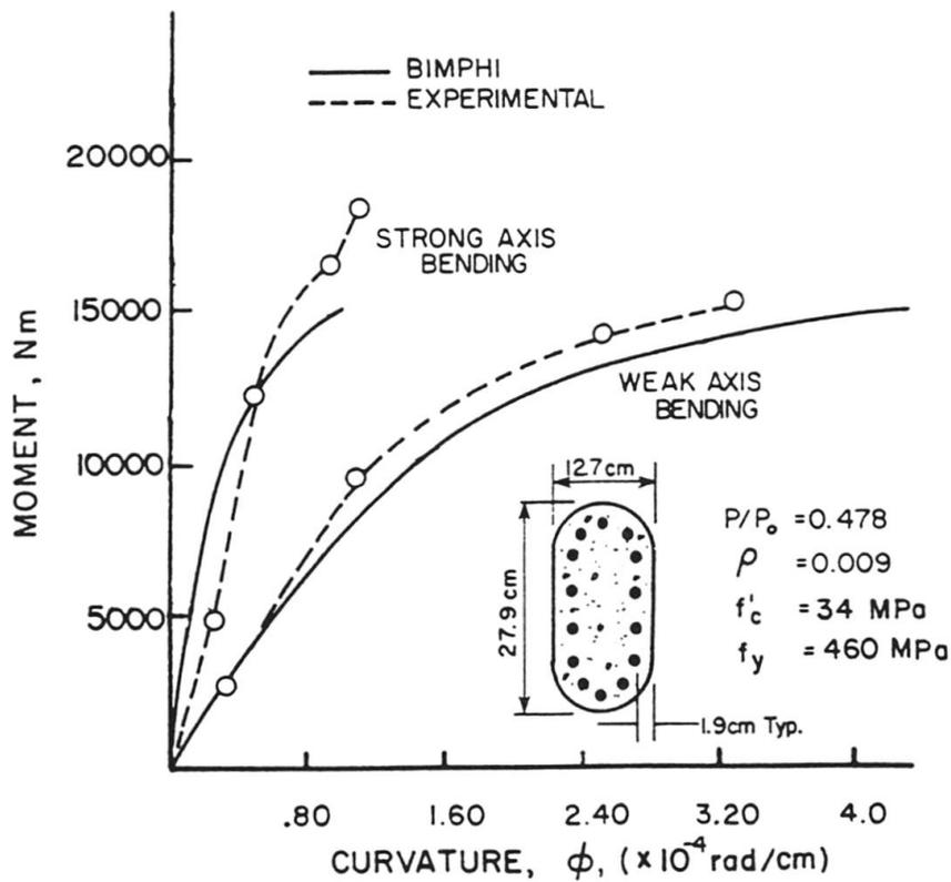
Fig. 2 Biaxial load-moment-curvature (P-M- $\phi$ ) relationship for solid oval section
