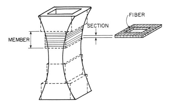
$\frac{\text{Fig. 1}}{\text{bridge pier}}$  Fiber model representation of a nonprismatic hollow
