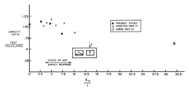
Fig. 7 Effect of wall thinness on pier capacity
