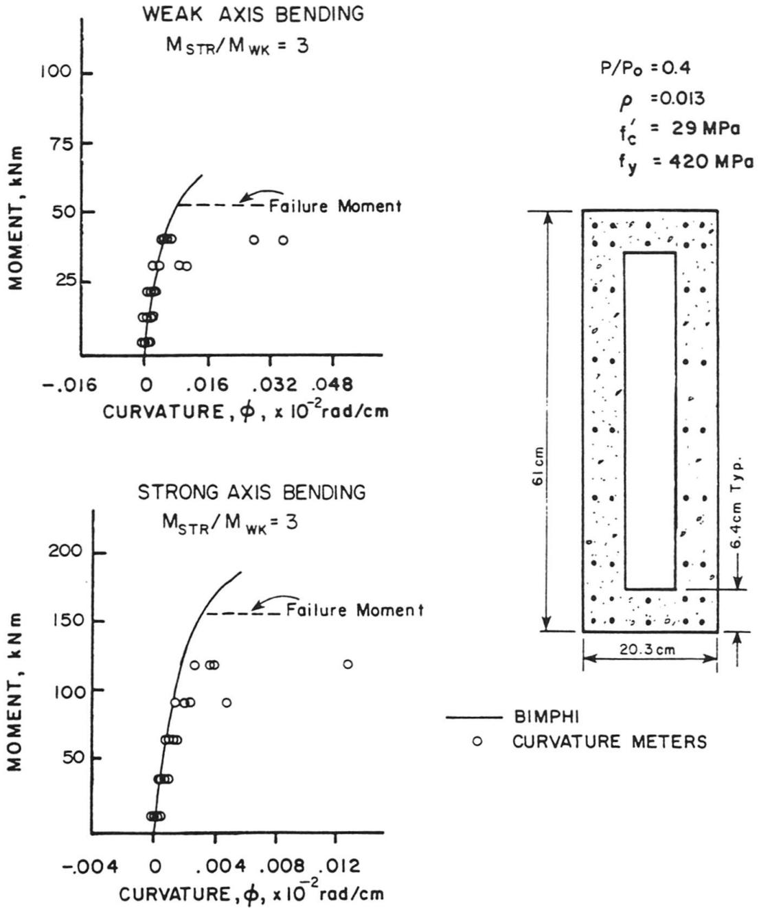
Fig. 5 P-M- $\phi$  behavior of single cell pier
