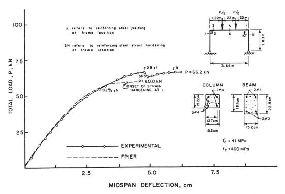
Fig. 4 Load-deflection behavior for reinforced concrete frame
