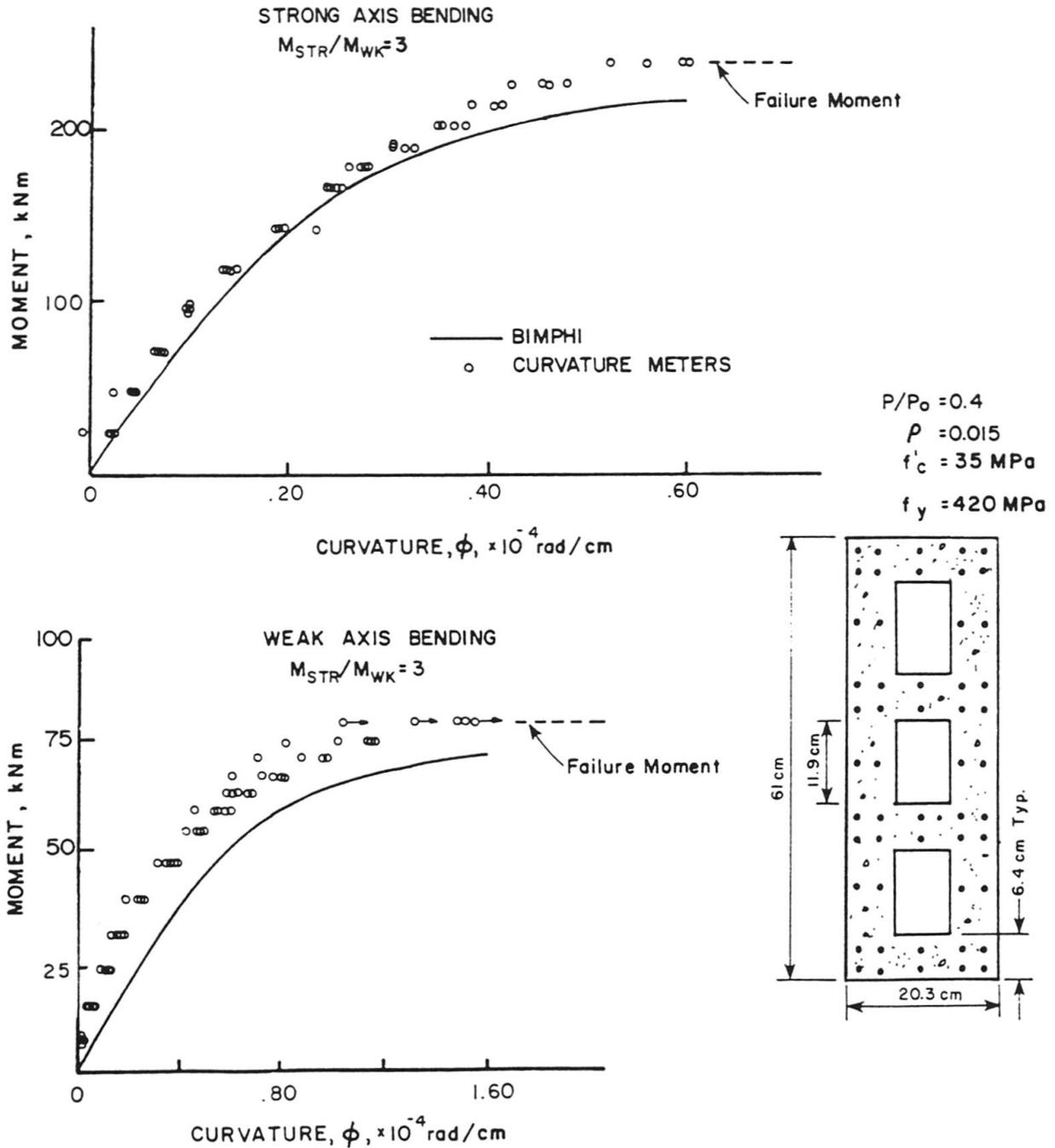
Fig. 6 P-M- $\phi$  behavior of three cell pier
