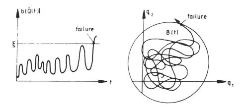
Fig.1 Geometrical illustration of failure event from combined load
