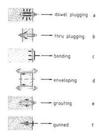
Fig. 13 Possiblities for Directing Tensile Forces into Existing Concrete
