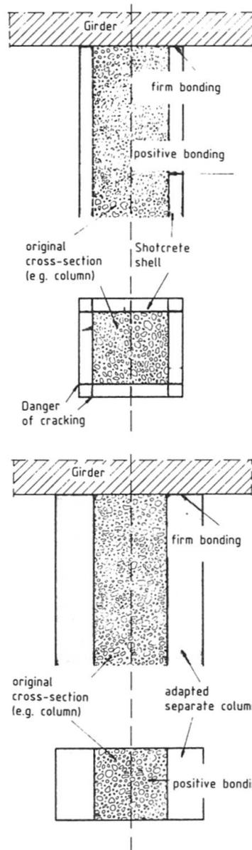
Fig. 11 Strengthening of a Column
