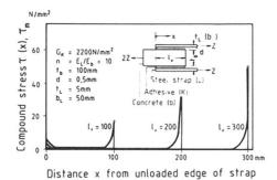
Fig. 14 Compound Stress Profile in the Bonded Joint of Bonded Steel Straps /4/
