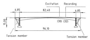
Fig. 7 Vibration System of Gänstor Bridge, on which Vibration Analysis was carried out according to Fig. 8
