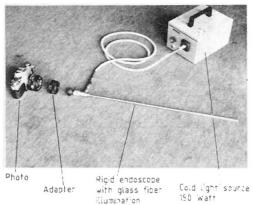
Fig. 3 Endoscope
