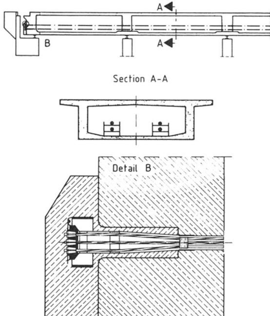
Fig. 15 Strengthening with Freely Guided Longitudinal Prestressing
