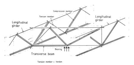
Fig. 10 Framework Analogy in Indirect Load Handling
