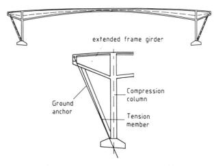
Fig. 19 Strengthening by Exterior Tension Members
