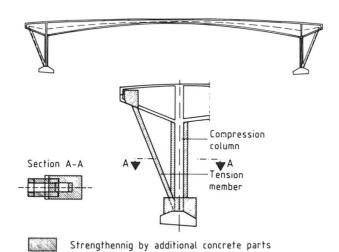
Fig. 20 Strengthening by Adapted Concrete Components
