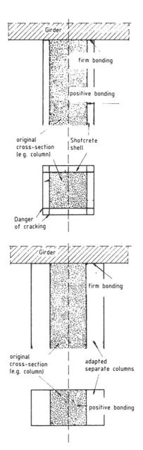
Fig. 11 Strengthening of a Column
