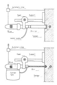
Fig. 2 Sensitive Drilling Technique
