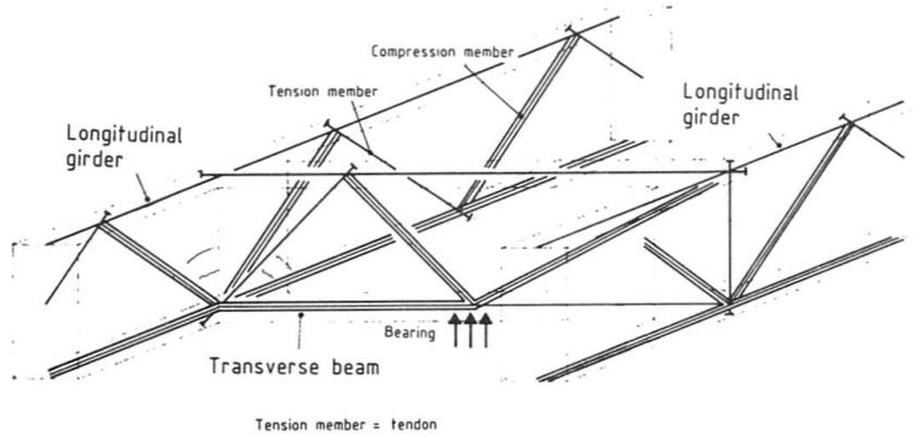
Fig. 10 Framework Analogy in Indirect Load Handling
