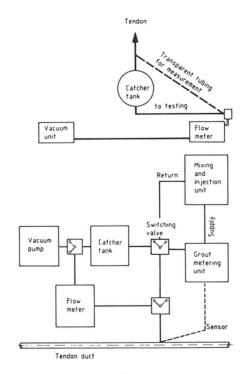
Fig. 4 Vacuum Method, Cavity Sensing, Grout Measurement
