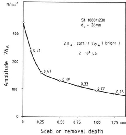
Fig. 6 Influence of Corrosion Scab on Fatigue Strength (26 mm dia St 1080/1230) /3/
