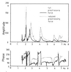
Fig. 8 Change of Frequency in the Bridge System as per Fig. 7
