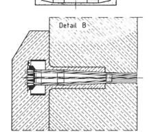
Fig. 15 Strengthening with Freely Guided Longi-tudinal Prestressing
