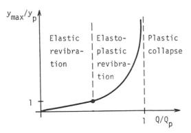
Fig. 3 Mid-deflection of a two-span beam subjected to loss of interior support
