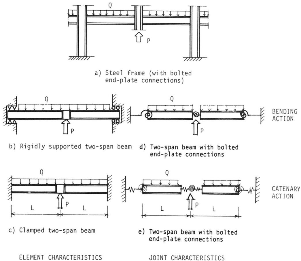
**Fig. 12.** Steel frame and its models
