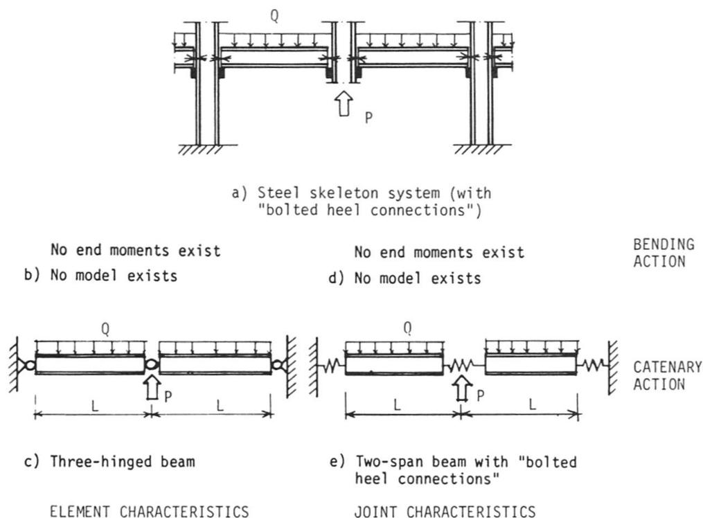
Fig. 13. Steel skeleton system and its models
