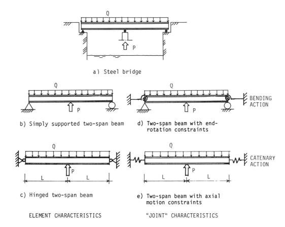
Fig. 11. Steel bridge and its models
