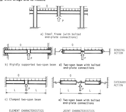
Fig. 12. Steel frame and its models
