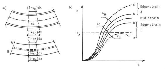
Fig. 6. Non-uniform compressive strain of the upper beam flange (a) and its time curve (b)
