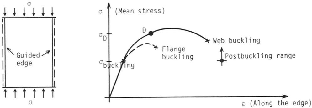
Fig. 5. Stress-strain curves for plates in compression
