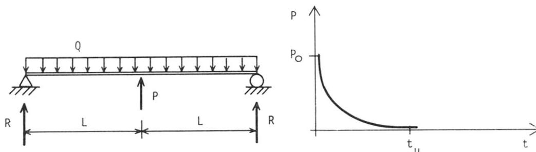
**Fig. 2.** Two-span beam subjected to removal of mid-support
