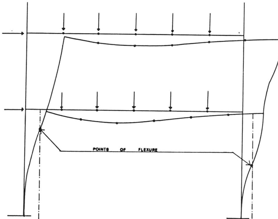
Fig.21 - Deformed shape of Example frame at Ultimate Limit State
