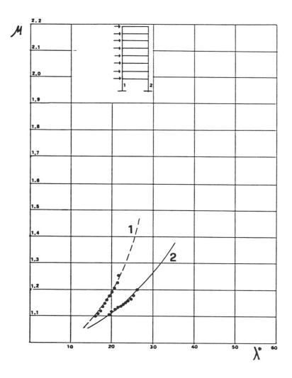
Fig. 22 -  ${\cal M}$  in ground floor columns of frame N.1 with increasing loads
