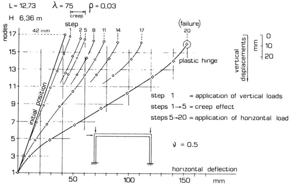
Fig. 14 - Displacements of left-hand column and beam
