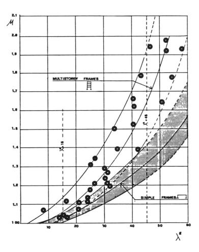
Fig.20 - Moment magnification factors in function of  $\lambda$  \* (Cauvin-Macchi expression).
