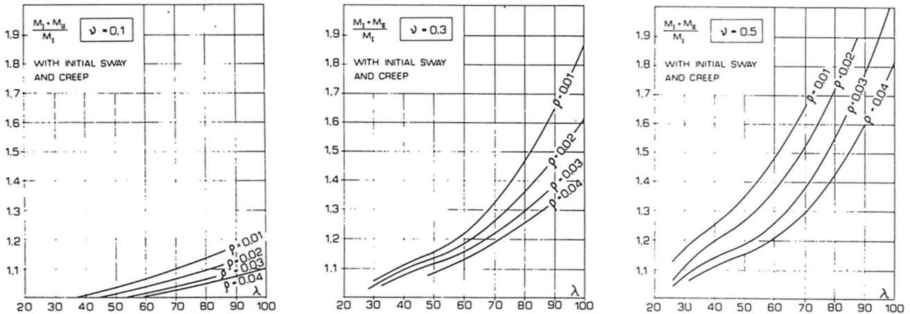
FIG. 25 - Moment magnification factors in function of  $\lambda$  and  $\nu$  for given values of  $\rho$ .
