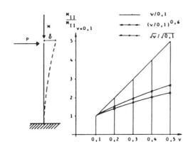
Fig.4 - Variation of M $_{ exttt{II}}$  in function of  ${oldsymbol {\mathcal V}}$
