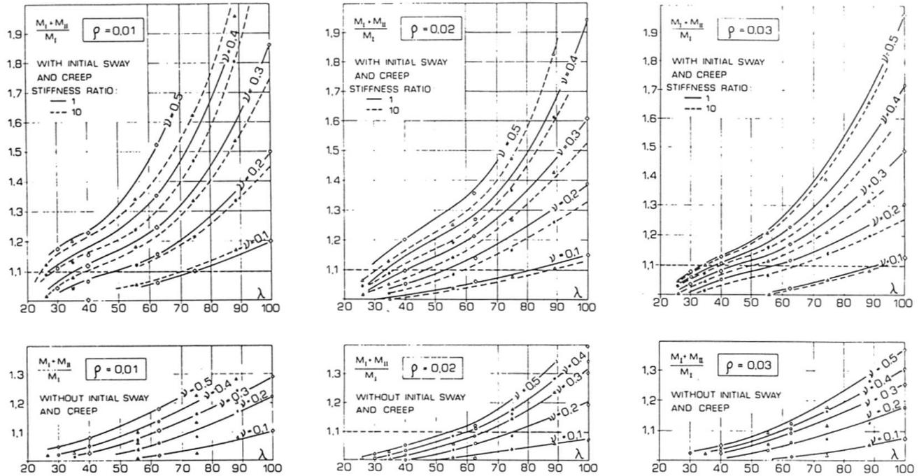
FIG. 24. Moment magnification factors in function of  $\lambda$  and  $\nu$  for given value of  $\rho$ .
