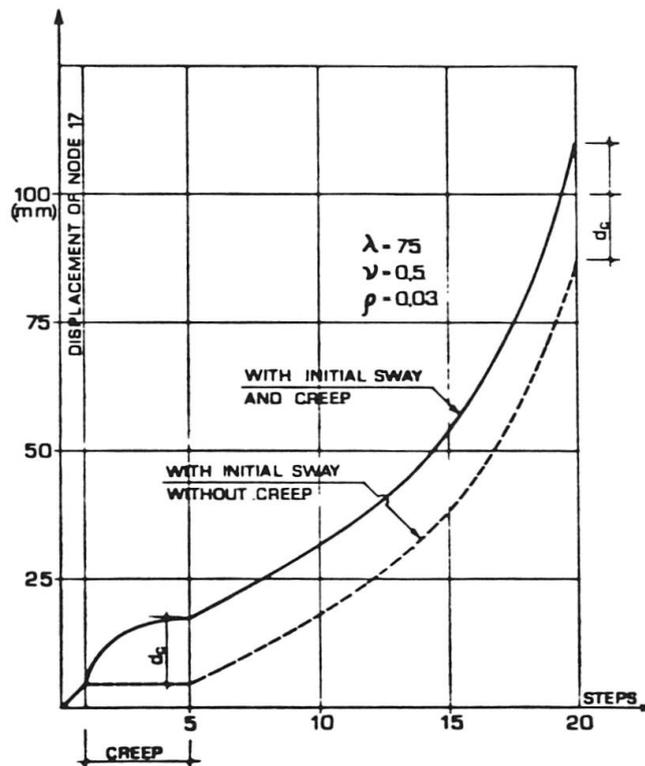
Fig. 15 - Displacements of upper joint of left-hand column for the two load histories
