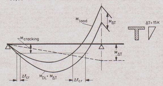
Fig. 8 Additional length  $\Delta \ell_{\rm cr}$  of the crack endangered zone of the bottom flange of a continous beam due to  $\Delta {\tt T}$
