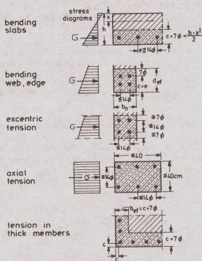
Definition of A<sub>c,eff</sub> for zones with different stress diagrams
