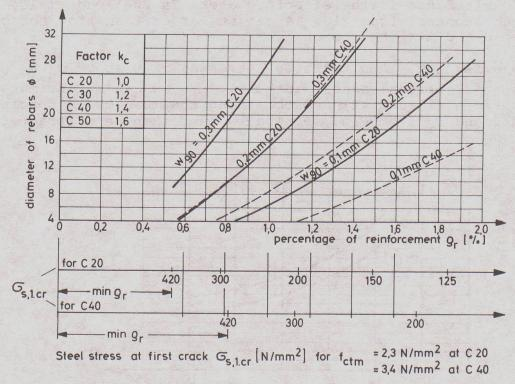
Fig. 14  $g_r$  - Ø diagram for axial tension, see text
