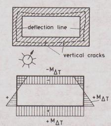
Fig. 6 Bridge pier, M due to sunshine by re-AT strained deformations
