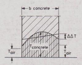
hardened concrete. However, quite often wide cracks show up due to these effects, even when much reinforcement was placed, because the young concrete gives not sufficient bond strength for making rebars effective to limit the crack width.
