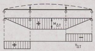
Fig. 3 Restraint action forces  $M_{\Delta T}$  and  $V_{\Delta T}$  at a continous beam due to  $\Delta T$
