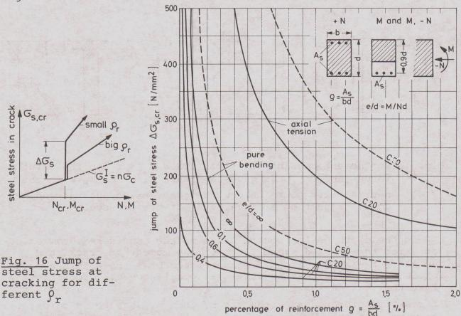
Fig. 17 Jump of steel stress  $\Delta \hat{\sigma}_{s,Cr}$  at cracking of concrete in a r.c.bar under tension + N or under bending by M or bending with longitudinal compression - N with different excentricity e/d, for  $f_{ct.m} = 0.19 f_{ck}^{2/3}$  [N/mm<sup>2</sup>].
