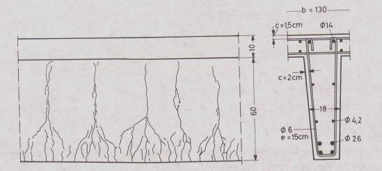
Fig. 12 Cracks of a T beam prove that the small crack spaces and the corresponding small crack widths obtained by the four bars  $\emptyset$  26 mm in the bottom flange are restricted to a small zone around the bars. Outside this zone, the web reinforcement was too weak to prevent wide cracks
