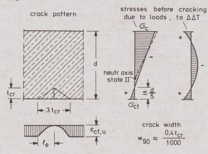
Fig. 19 If  $\mathcal{E}_{\rm ct} <$  0,015 % then crack width remains small without reinforcement
