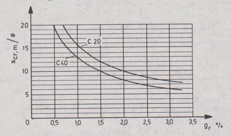
Fig. 15 Mean crack spaces  $s_{\rm cr,m}$  at a r.c.bar under tension, related to bar  $\emptyset$  and  $\mathcal{G}_{\rm r}$
