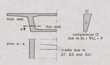
Fig. 5 Transverse cracks in thin bottom slab due to  $\Delta S$ ,  $\Delta Cr$ ,  $\Delta T$  in spite of high prestressing
