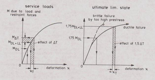
Fig. 9 Priestley's display how restraint forces MAT disappear in hyperstatic structures due to cracking and plastic deformation if loads are increased to the ultimate limit state, here full prestressing for load moments.
