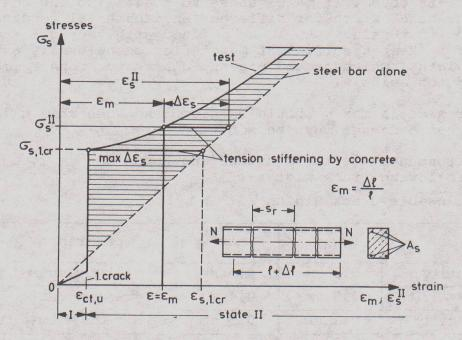
Fig. 11 Stress-strain diagram of a reinforced concrete bar under axial tension. Definition of the & values for crack width formulae
