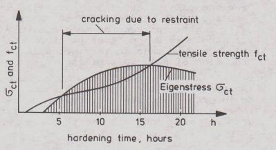
Fig. 1 Heat of hydration gives high temperature T. Cooling from outside causes "Eigenstresses"
