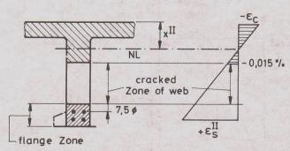
Fig. 7 Cracking zone in webs of beams under max M load DL+ LL+restraint
