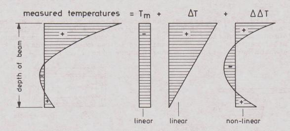
Fig. 4 Division of a temperature diagram into linear ΔT and non-linear ΔΔT
