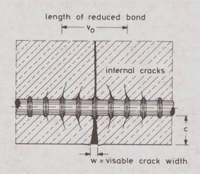
of research [7] and [8] and experience showed that crack widths up to w = 0,4 mm do not significantly harm the corrosion protection of the rebars, if the concrete cover is sufficiently thick and dense.
