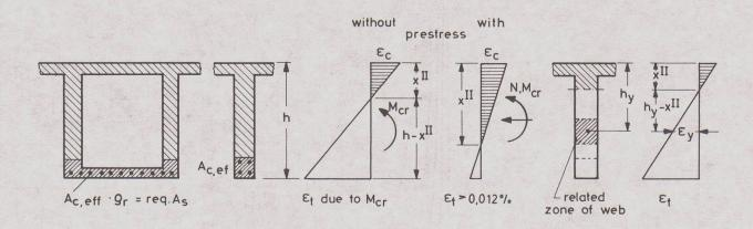
Fig. 18 The moment causing the first crack  $M_{\rm Cr}$  due to restraint forces and/or loads gives a strain diagram  $\mathcal{E}_{\rm C}$  with the neutral axis at  ${\rm X}^{\rm II}$  below the compressive edge depending on the amount of  ${\rm A_S}$  or  ${\rm A_S}$  +  ${\rm A_p}$  if prestressed.
