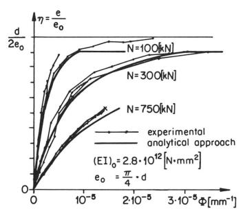
Fig.7 Calibration of  $\eta$ - $\Phi$  Curves
