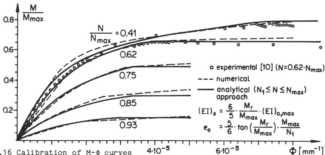
Fig.16 Calibration of M- $\phi$  curves
