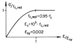
Fig.14 Concrete Stress-Strain Relationship
