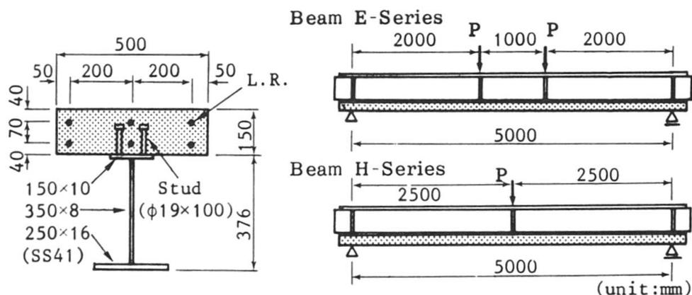
Fig. 1 Cross-section and loading points of beam specimens.
