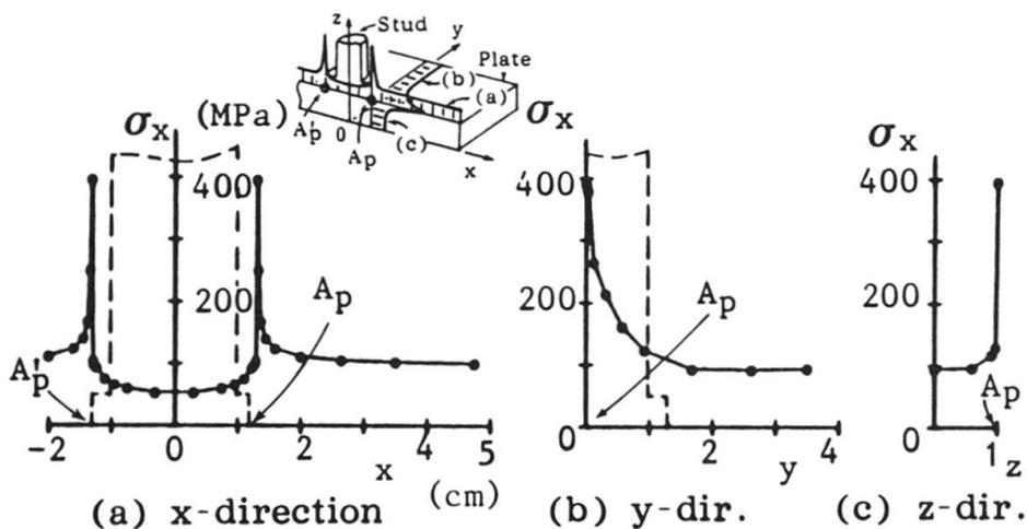
Fig. 12 Stress distributions under tension only.
