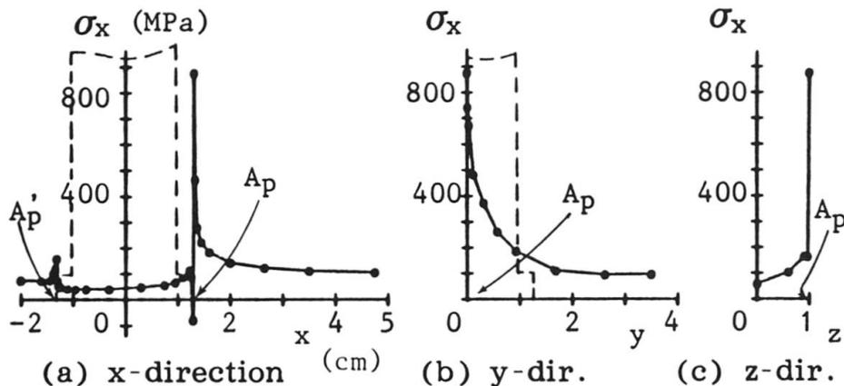
Fig. 15 Stress distributions under combined tension and shear.
