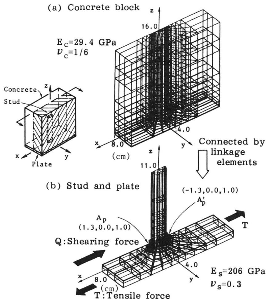
Fig. 10 Finite element mesh division.
