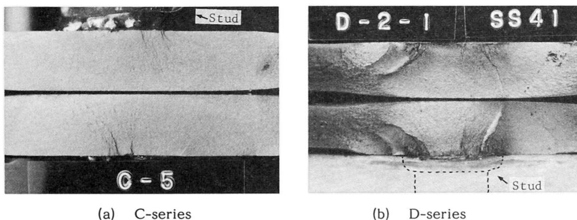
Fig. 9 Typical fracture surface of coupon specimens.
