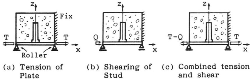
Fig. 11 Loading and boundary conditions.
