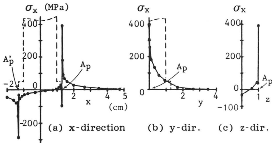
Fig. 13 Stress distributions under shear only.
