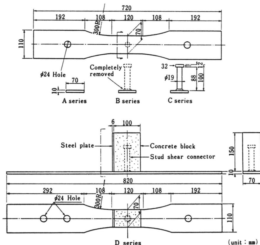
Fig. 4 Coupon specimens.
