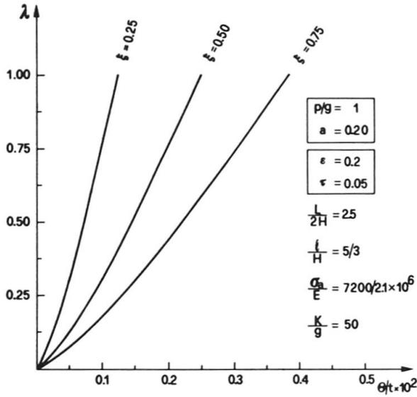
Fig. 7 Continuous model: midspan torsional rotation ( $\epsilon=0.2, \tau=0.05$ ).
