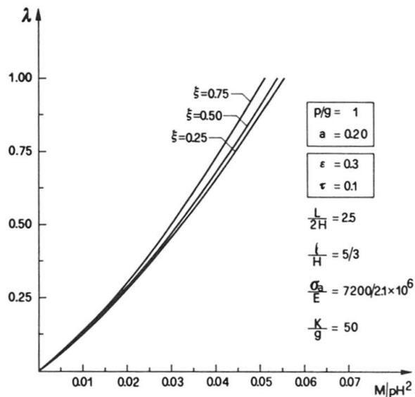
Fig. 6 Continuous model: midspan bending moment ( $\epsilon=0.3, \tau=0.1$ ).
