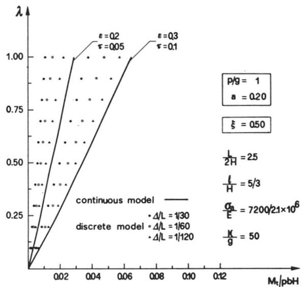
Fig. 14 Twisting moment at the section  $\zeta=0$ : comparison between analytical and numerical results.
