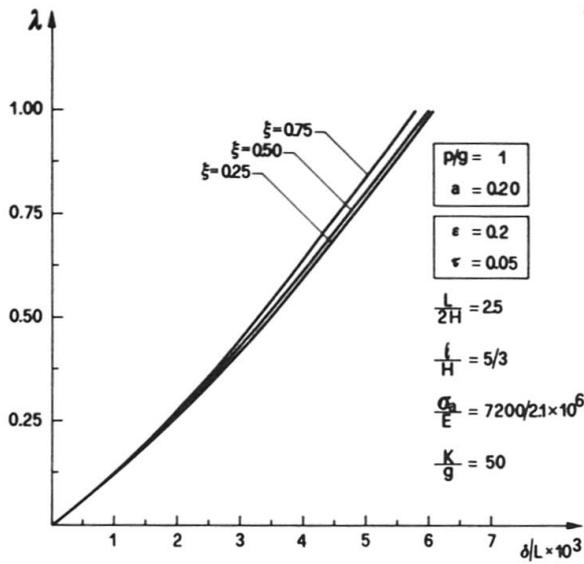
Fig. 3 Continuous model: midspan deflection ( $\epsilon=0.2, \tau=0.05$ ).
