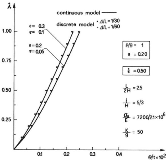
Fig. 13 Midspan torsional rotation comparison between analytical and numerical results.
