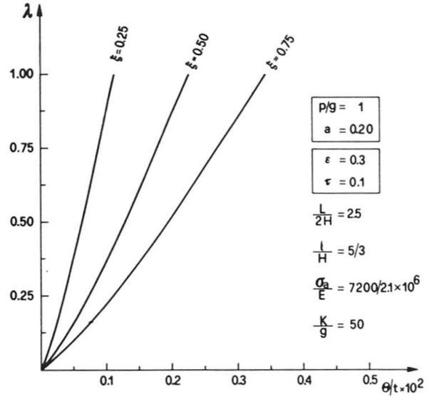
Fig. 8 Continuous model: midspan torsional rotation ( $\epsilon=0.3, \tau=0.1$ )
