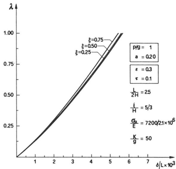
Fig. 4 Continuous model: midspan deflection ( $\epsilon=0.3, \tau=0.1$ ).
