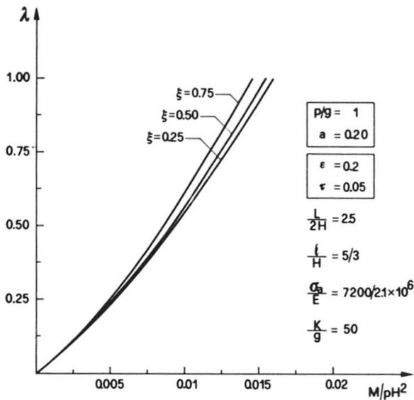
Fig. 5 Continuous model: midspan bending moment ( $\epsilon=0.2, \tau=0.05$ ).
