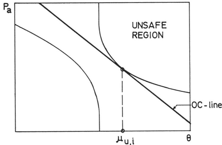
Fig.15 Location of the mean value of the process curve in the most unfavourable case
