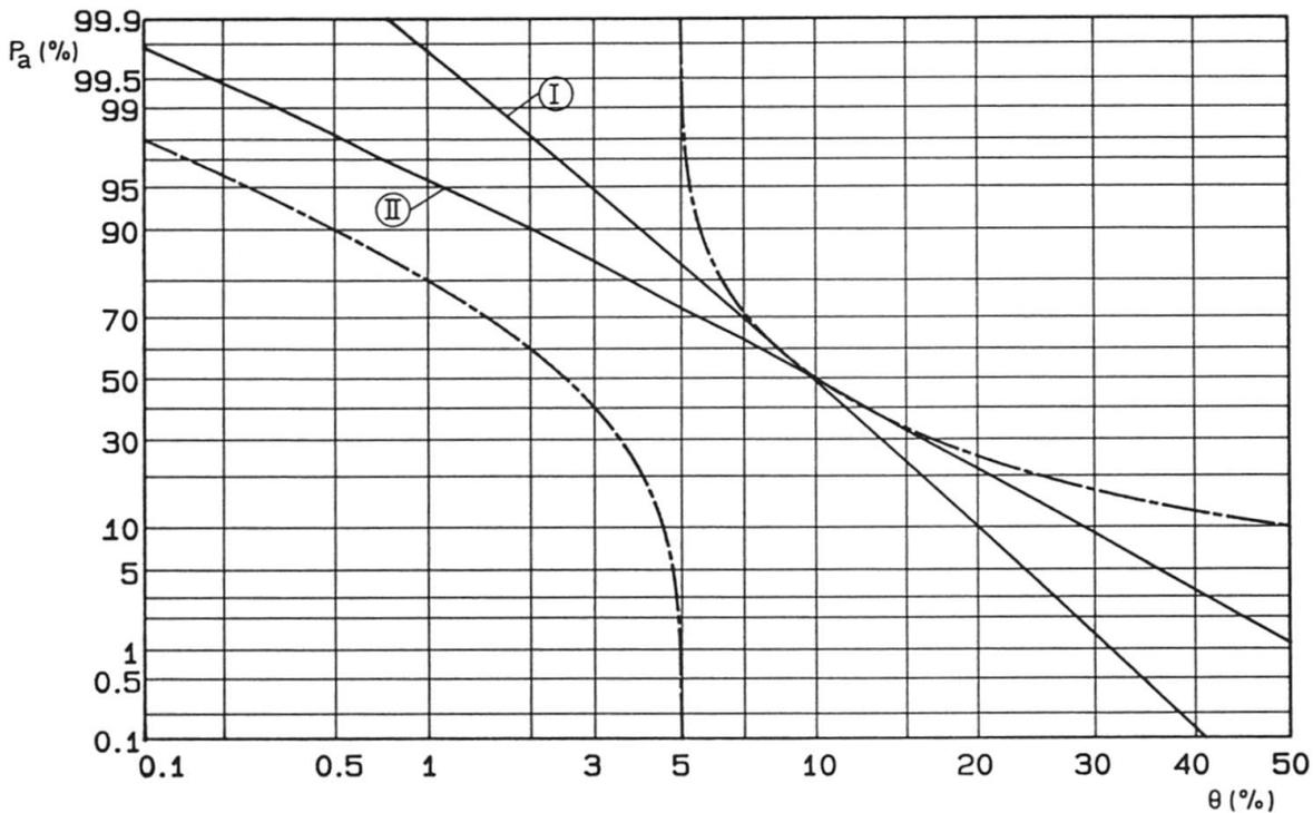
**Fig.13** Criterion  $\bar{x}_{15} \geq f_{ck} + \lambda s_{15}$  ( $\lambda$  according to table 2). OC-lines tangent to the unsafe region. Independent observations (I); AR(2)-model (II)
