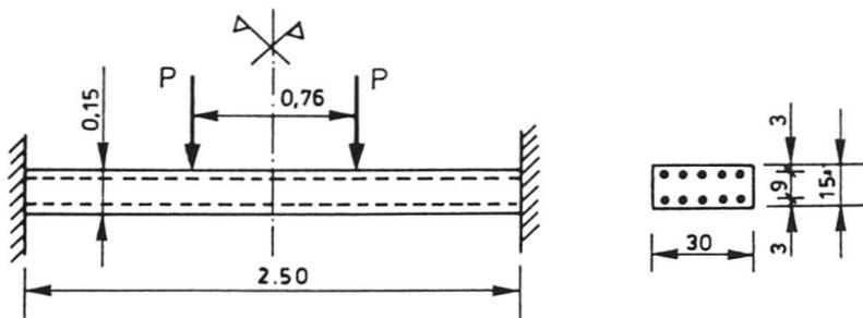
Only rotational restraint was imposed at both ends; the slab was free to expand axially.
