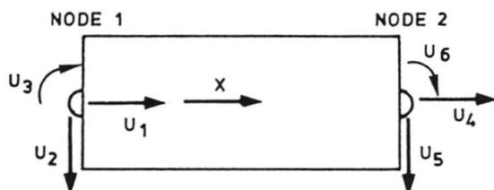
The midplane axial displacement is linear, whereas the lateral displacement is a cubic function of  $x$ . The Navier-Bernoulli hypothesis is respected and the shear energy is not taken into account.
