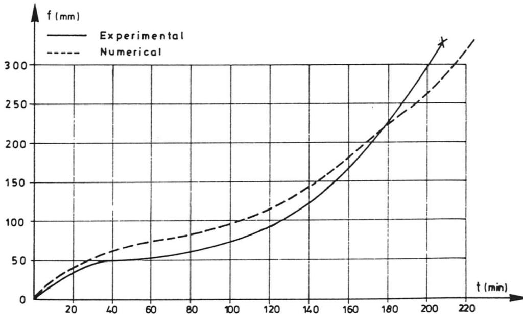
Fig. 10 Deflection versus time curve at mid-point
