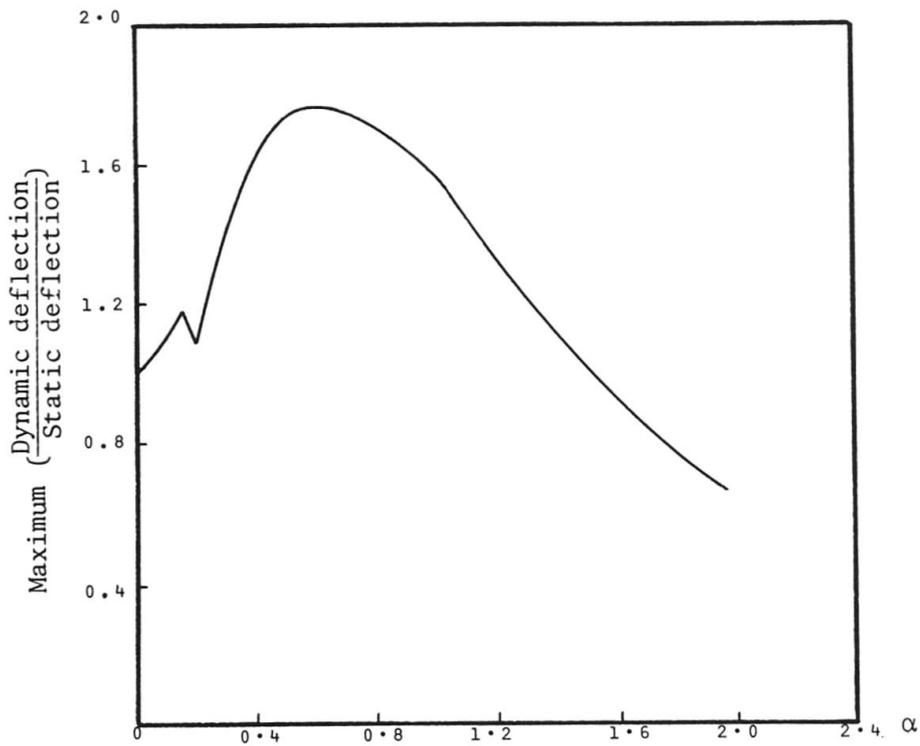
Fig. 7 Maximum dynamic influence line values for mid-span deflection versus speed parameter  $\alpha$ .
