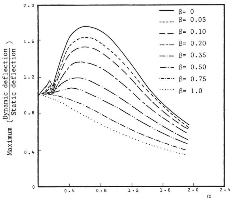
Fig. 9 Maximum dynamic influence line values for mid-span deflection versus speed parameter  $\alpha$  with various damping values.
