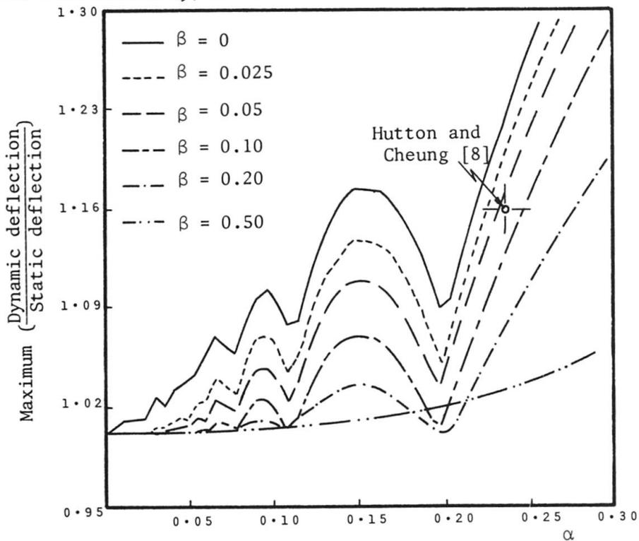
Fig. 8 Maximum dynamic influence line values for mid-span deflection versus speed parameter  $\alpha$  with various damping values.
