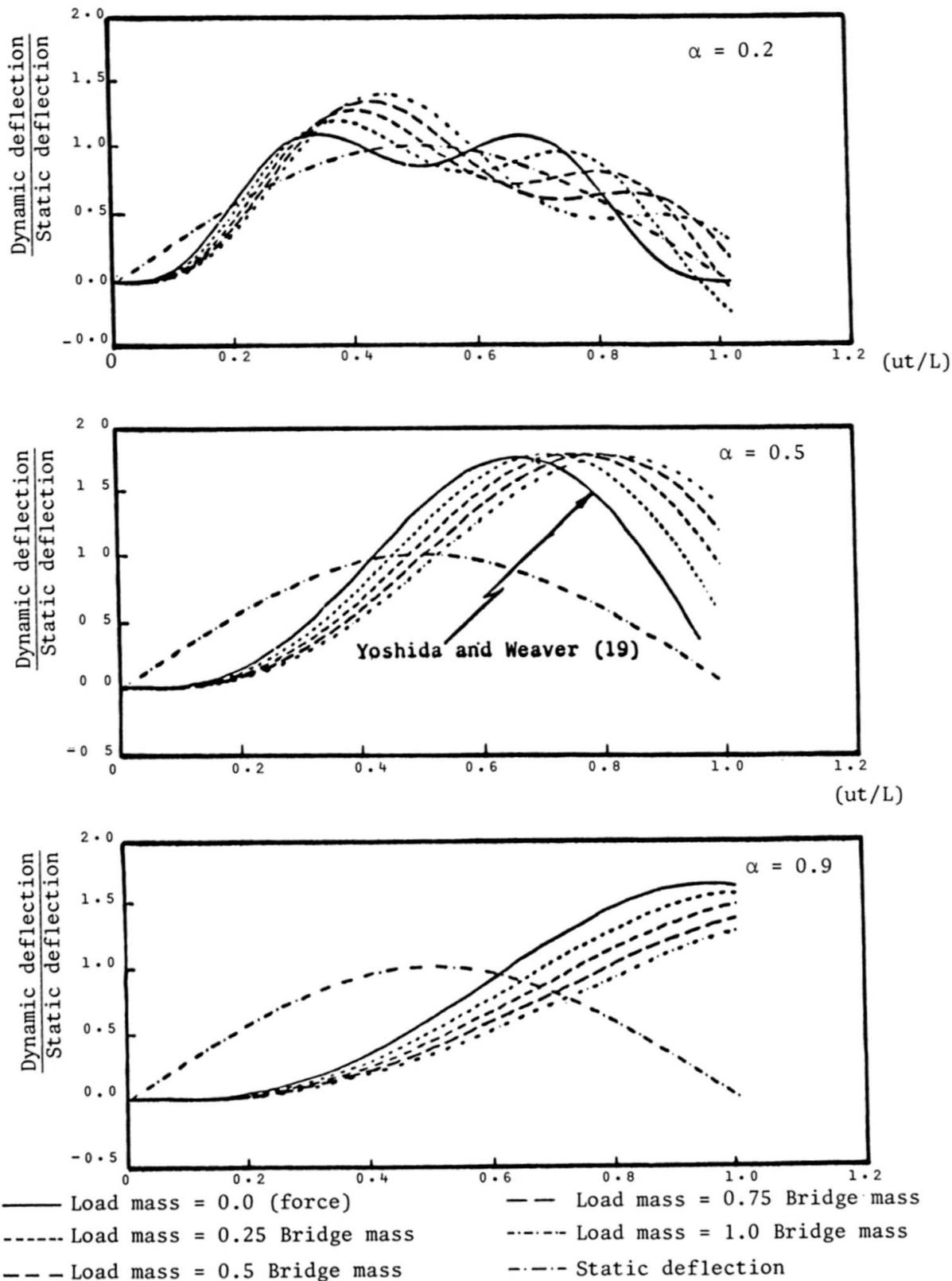
Fig 2 Comparison between dynamic influence lines for mid-span deflection of a moving force and a moving mass with various mass ratios. (Mass ratio = mass of load/mass of bridge) Speed parameter  $\alpha = 0.2, 0.5, 0.9$ .  $\beta = 0$
