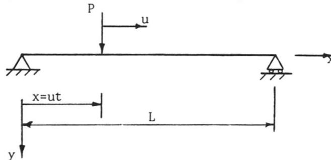
Fig. 1 Moving load on a simply supported beam
