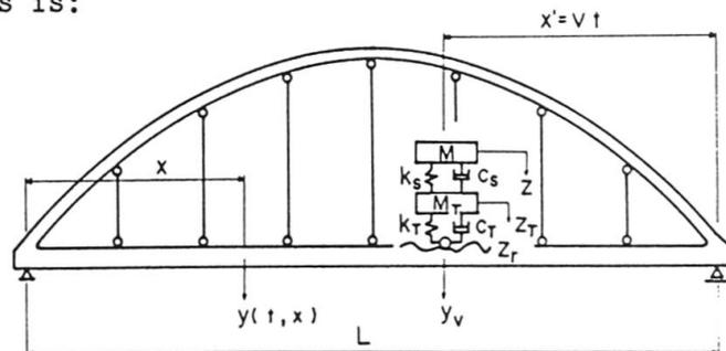
Fig.3 Vehicle-bridge system.
