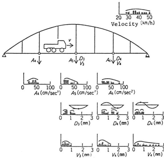
**Fig.11** Maximum response values (reinforcement not applied; 12 case).
