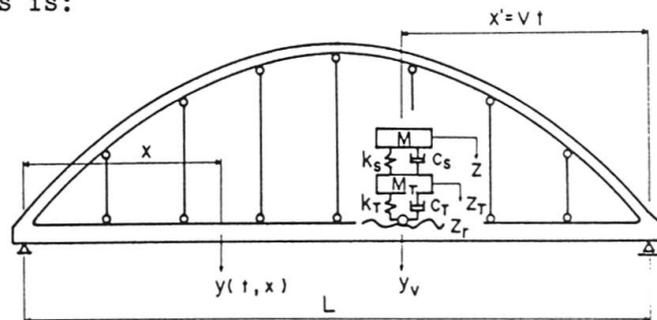
Fig.3 Vehicle-bridge system.
