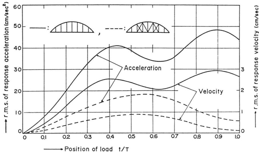
Fig.8 Relation between structural systems and effective values.
