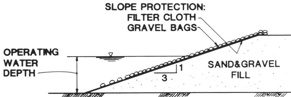
Fig. 3 Typical Cross-Section, Sandbag-Retained Artificial Gravel Island
