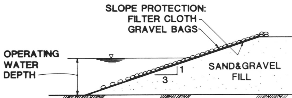
Fig. 3 Typical Cross-Section, Sandbag-Retained Artificial Gravel Island
