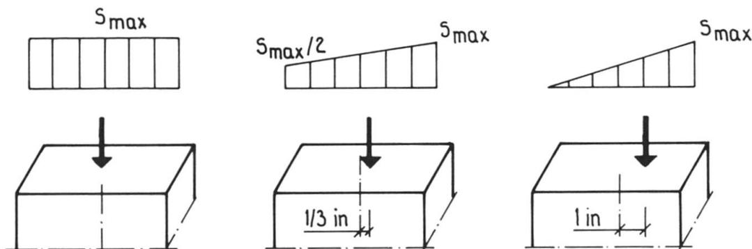
Fig 8 Stress gradients used in a fatigue experiment [9].
