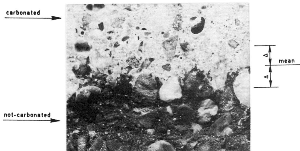
Fig. 7 Irregular carbonation front in concrete
