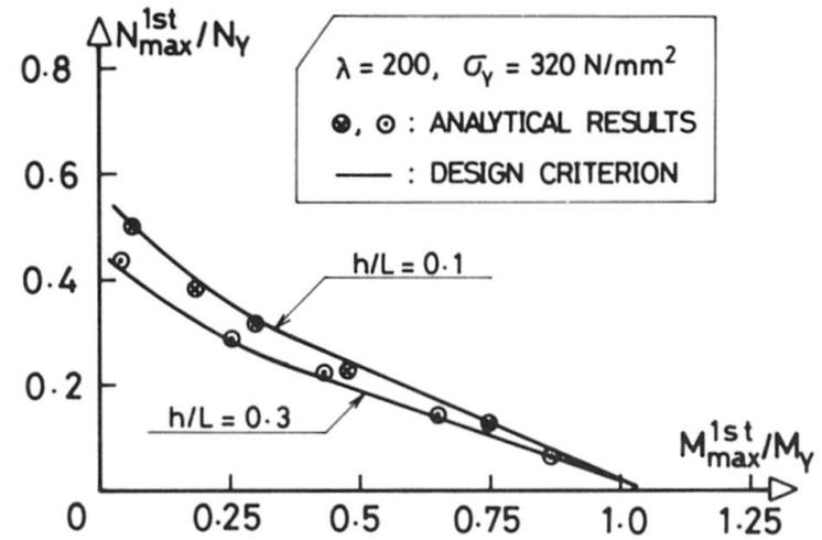
Fig.2 Relationship Between Maximum Thrust & Bending Moment
