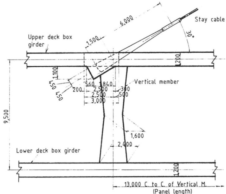
Fig. 5 Anchorage of stay cable (unit in mm)
