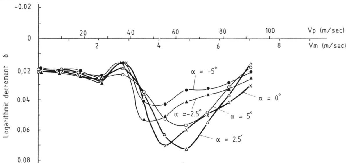
Fig. 18 Aerodynamic damping,  $V-\delta$  curves
