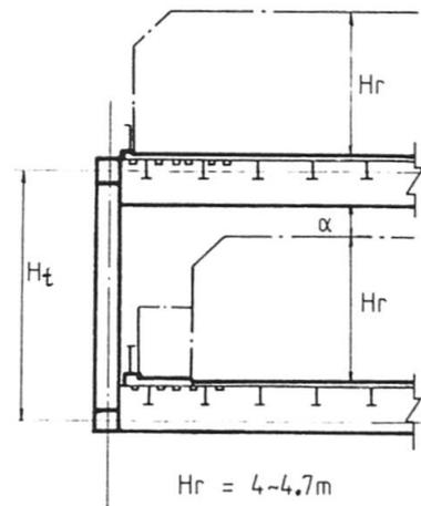
Fig. 1 Construction gauge of double deck bridge
