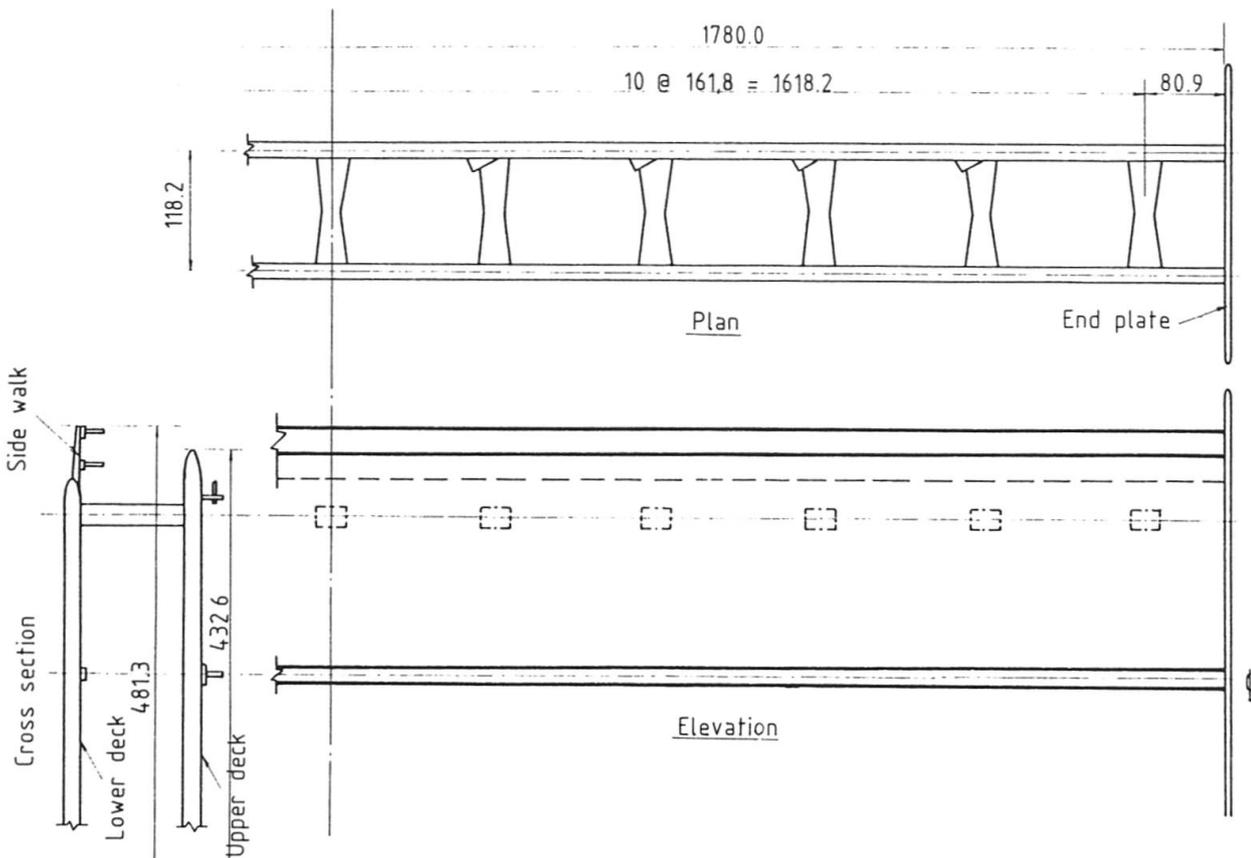
Fig. 10 General view of section model of Vierendeel-type (unit in mm)
