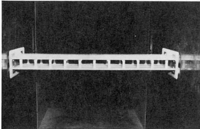
Photo 2 Two-dimensional section model in wind tunnel
