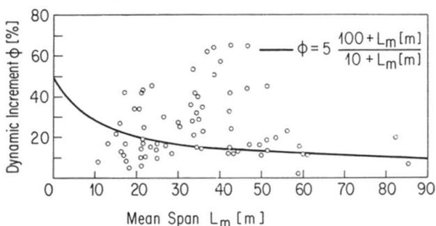
Fig. 15 Dynamic increments  $\phi$  for passages without a plank as a function of the mean span  $L_m$ . 73 values of concrete bridges,  $\alpha \leq 0.8$ . The solid line indicates the relation given in [7].
