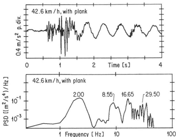
**Fig. 20** Time signal and PSD-spectrum of acceleration (AC14).
