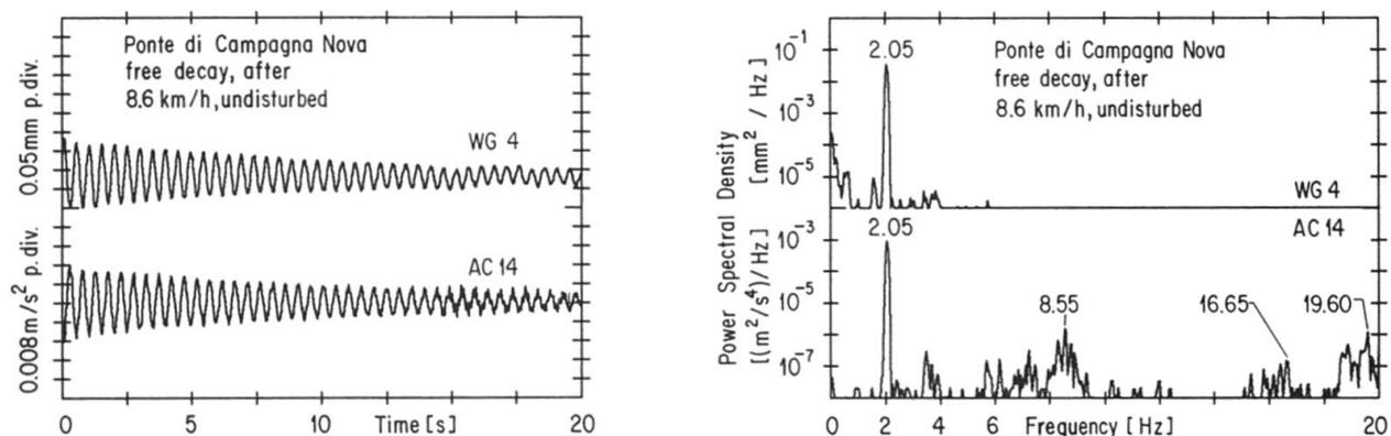
**Fig. 18** Time signals and PSD-spectra of displacement (WG4) and acceleration (AC14) measured at the mid-point of the Ponte di Campagna Nova at a parapet. The frequencies of the modes having non-zero amplitudes at the measurement point are indicated.
