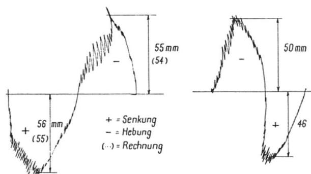
**Fig. 2** Kettenbrücke Aarau (one suspended 97.5 m span); dynamic load tests of 1922. Deflection traces measured and recorded with a vibrograph (from [1]). Left: Passage of 70 riders with a total mass of 42 t at a normal pace. Right: Passage, in the reverse direction, of 12 riders with a total mass of 7.2 t at a trot.
