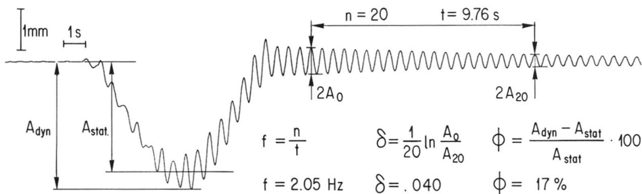
**Fig. 7** Deflection of the mid-point of the Ponte di Campagna Nova (one 45 m-span) under the passage of a 160 kN vehicle with  $v = 25$  km/h on the undisturbed pavement.  $f$  = fundamental frequency,  $\delta$  = logarithmic decrement,  $\phi$  = dynamic increment.
