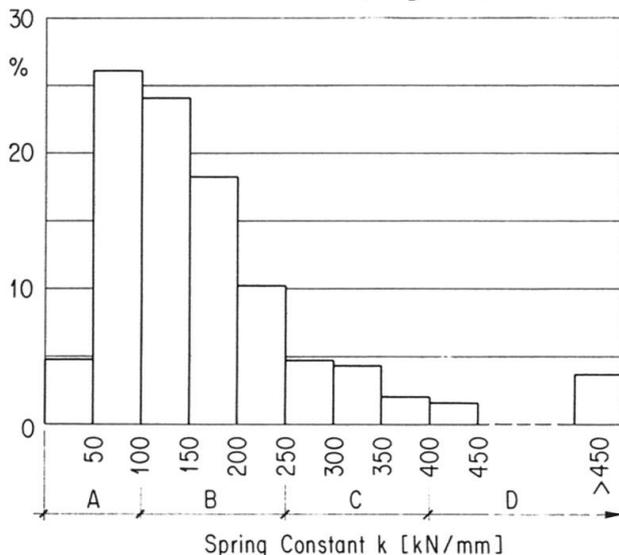
**Fig. 10** Spring constant  $k$  of the bridges. 187 values; min.: 7 kN/mm, mean: 173 kN/mm, max.: 800 kN/mm. Classification of the flexural stiffness of a bridge: A: flexible, B: average, C: stiff, D: very stiff.
