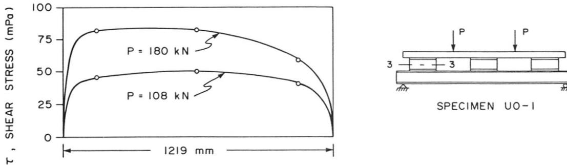
Fig.7 Shear stress distribution across section 3-3
