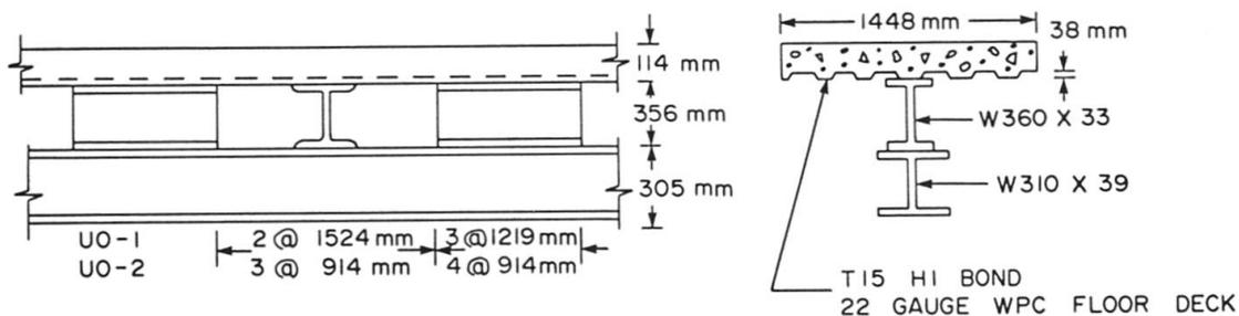
Fig.3 Specimen dimensions
