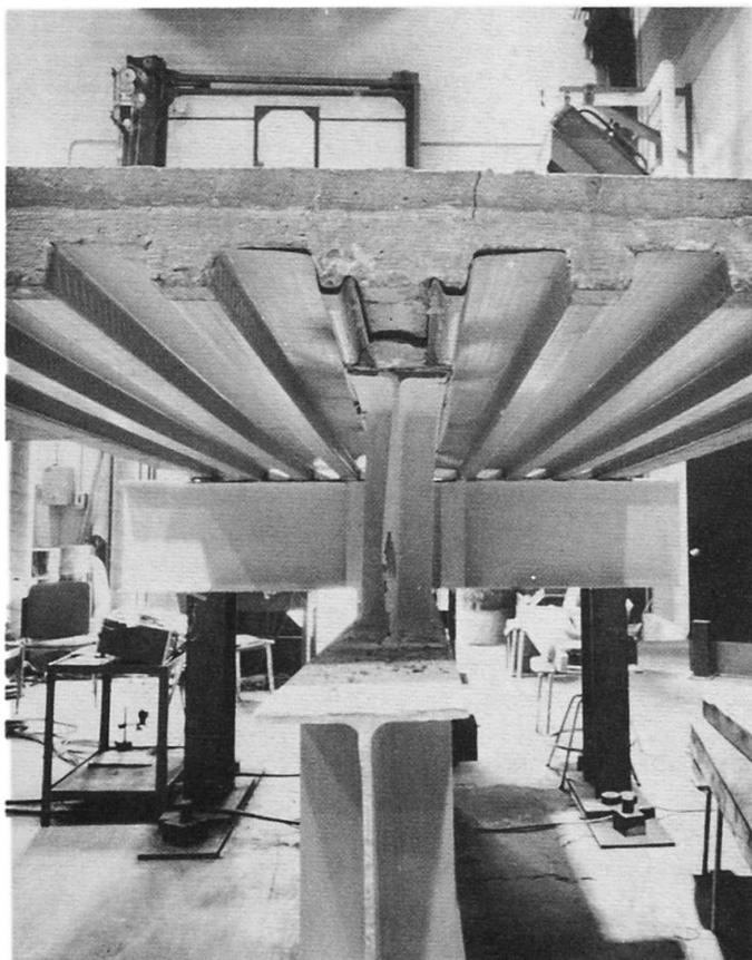
Fig.6 Slab failure region over the end stub
