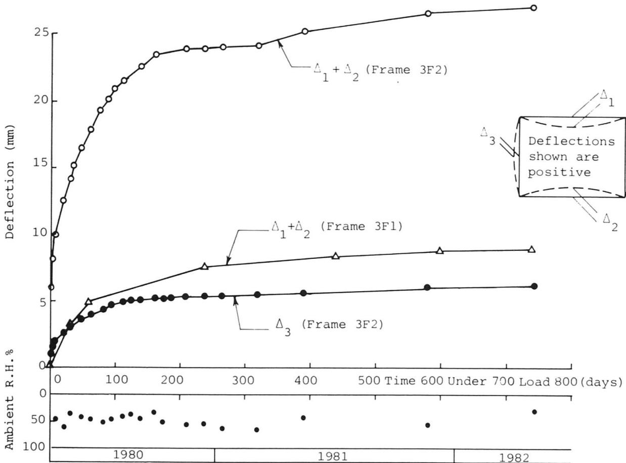
Fig. 7 Midspan deflections of frames 3F1 and 3F2
