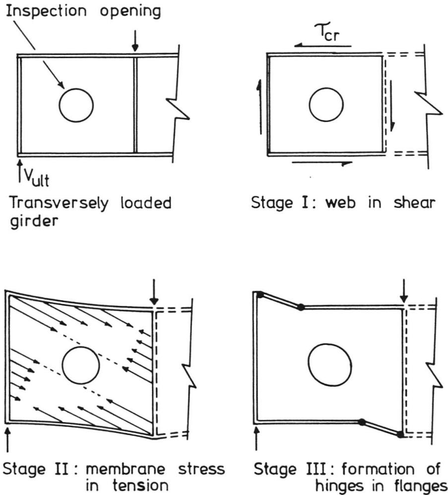
FIG. 1 FAILURE MECHANISM
