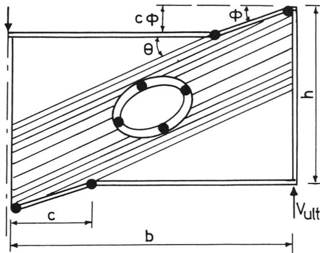
FIG.4 WEB WITH REINFORCED HOLE UNDER SHEAR LOADING
