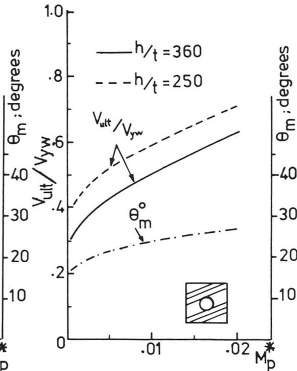
FIG. 2(b) PANEL OF ASPECT RATIO 1 HAVING A CUTOUT  $d/h = 0.3$
