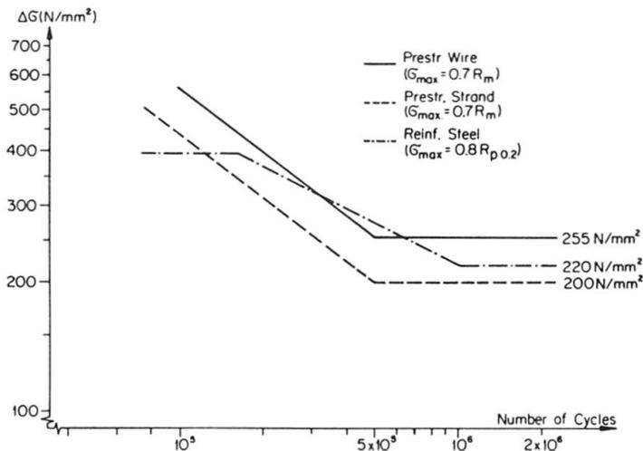
Fig. 3: Fatigue Strength of Reinforcing and Prestressing Steels
