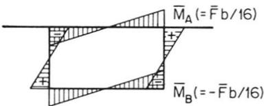
Fig. 8: Box Section, Transverse Bending
