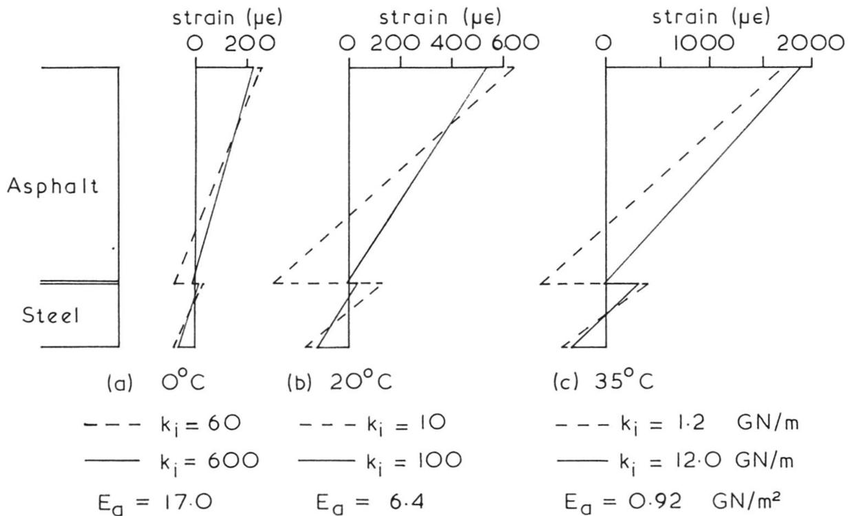
Fig.11. Effect of Variation in Tack Coat Stiffness
