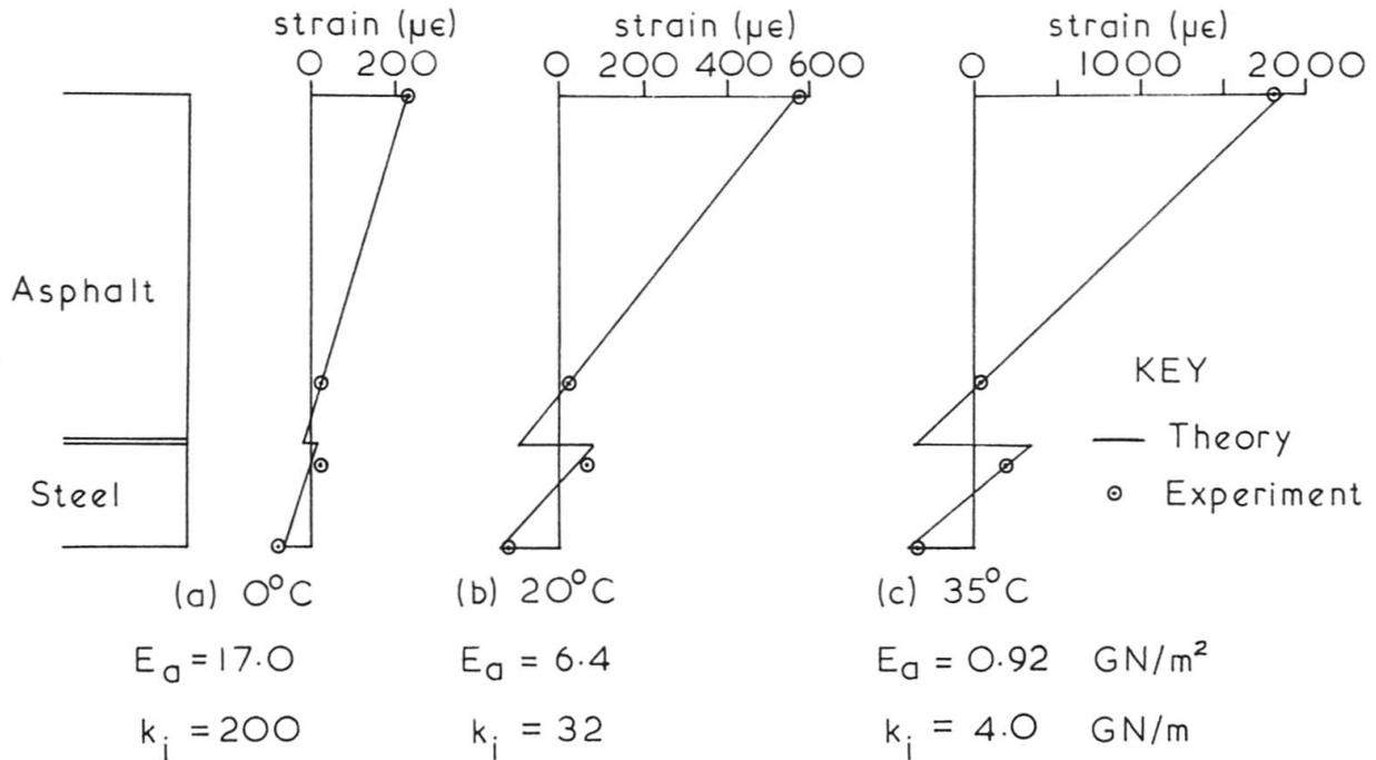
Fig.10. Experimental Strains Compared with Stress Function Theory
