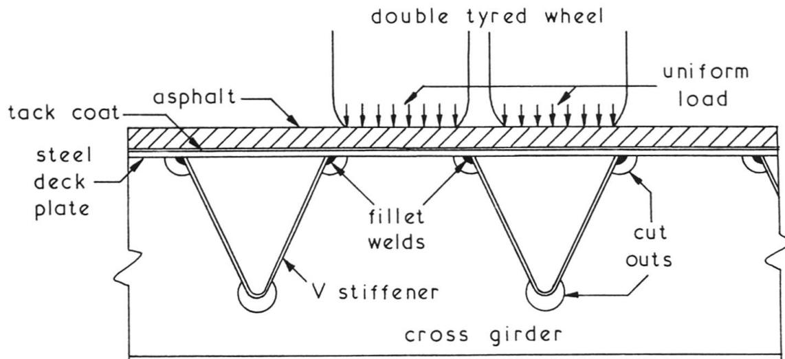
Fig.1. Orthotropic Steel Bridge Construction
