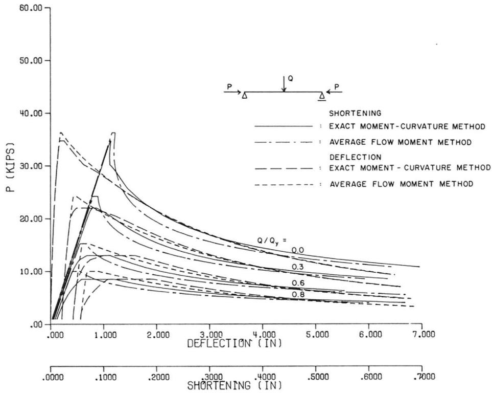
Fig.16 Comparison between Exact Moment-Curvature Method and Average Flow Moment Method, Pin-Ends,  $L/r=80$
