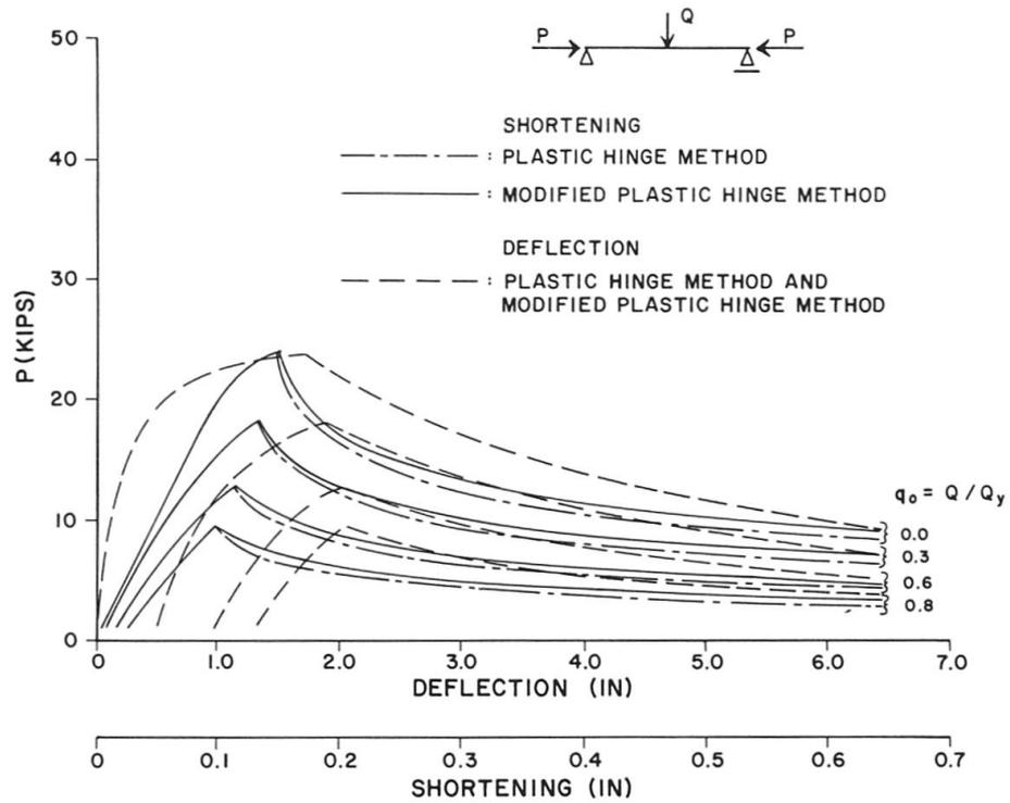
Fig.7 Comparison between Plastic Hinge Method and Modified Plastic Hinge Method, Pin-Ends,  $L/r=120$
