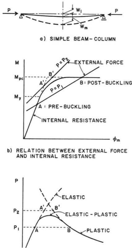
Fig.1 General behavior of a Beam-Column
