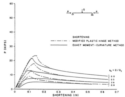
Fig.10 Comparison between Exact Moment-Curvature Method and Modified Plastic Hinge Method, Pin-Ends, L/r=80
