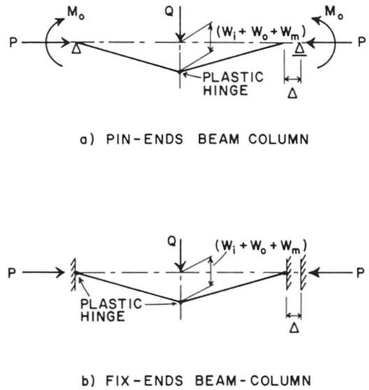
Fig.4 Plastic Hinge Method
