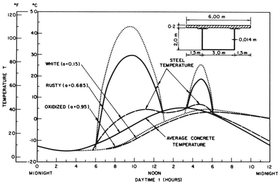
Fig. 15 Diurnal Variation of Maximum Temperature in Steel Box and Average Temperature in Concrete Deck for Different Absorptivities of the Steel Surface (Spring Conditions,  $\gamma = 45^\circ$ )
