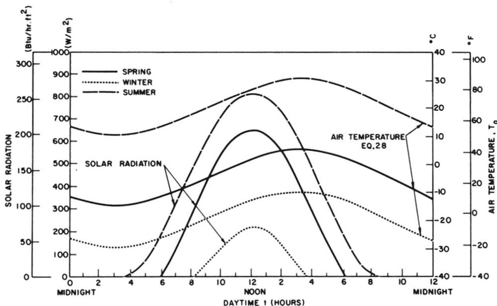
Fig. 8 Idealization of Diurnal Variation of Ambient Air Temperature and Solar Radiation Intensity Received on a Horizontal Surface for Different Seasons (Conditions at Calgary, Canada)
