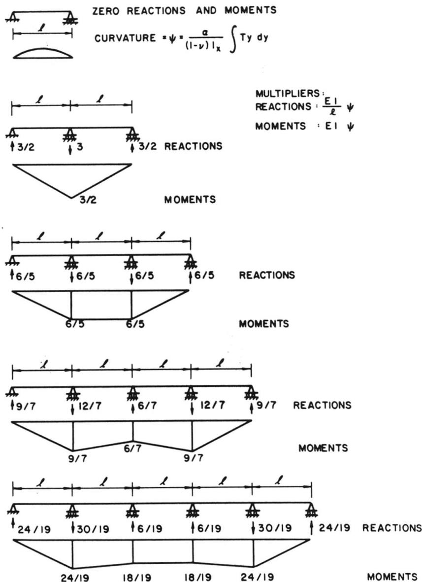
Fig. 7 Reactions and Bending Moments in Continuous Beams due to Temperature Rise (See Fig. 5)
