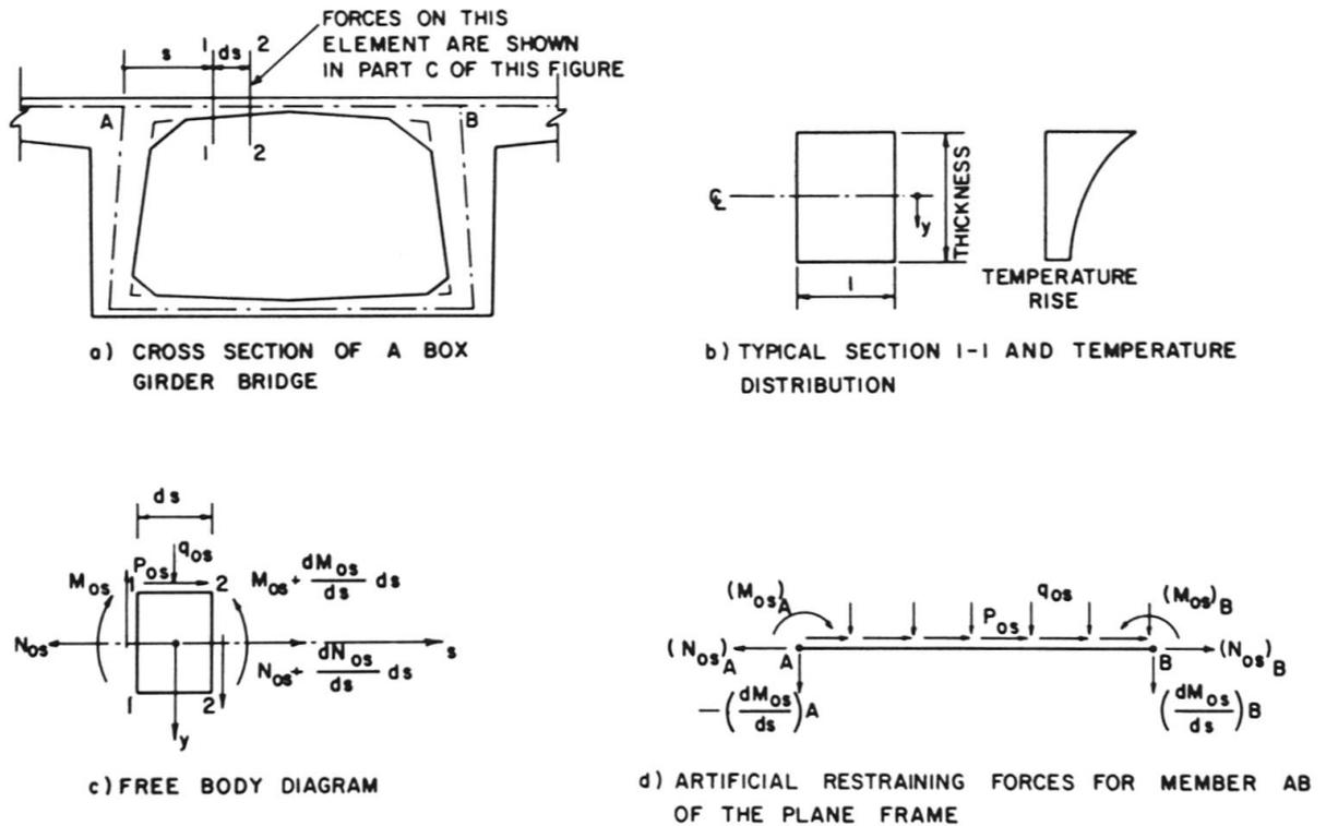
Fig. 4 Calculation of Stresses in Transverse Direction
