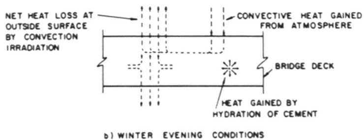
Fig. 1 Heat Gain and Loss Processes
