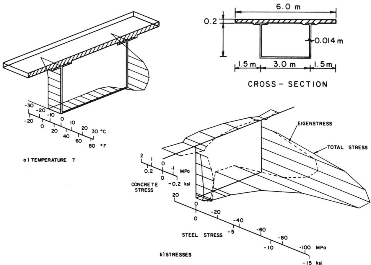
Fig. 10 Temperature and Eigen and Total Stress Distributions in a Section at the Central Support of a Two-Span Continuous Composite Box-Girder Bridge (Winter Conditions in Calgary, Canada,  $\gamma = 0^{\circ}$ )
