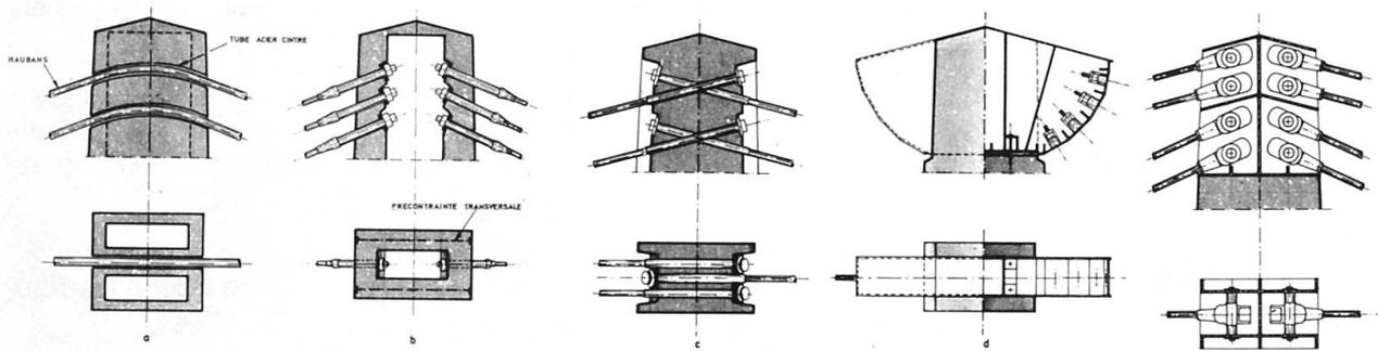
Figure 2 - Connection of cable stays to towers
