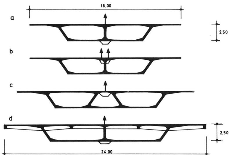
Figure 3 - Multicell box girders
