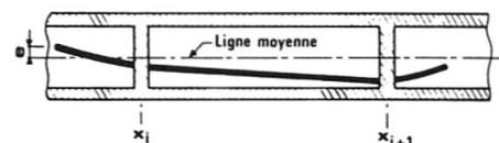
Figure 6 - External tendon over-stressing : calculation data
