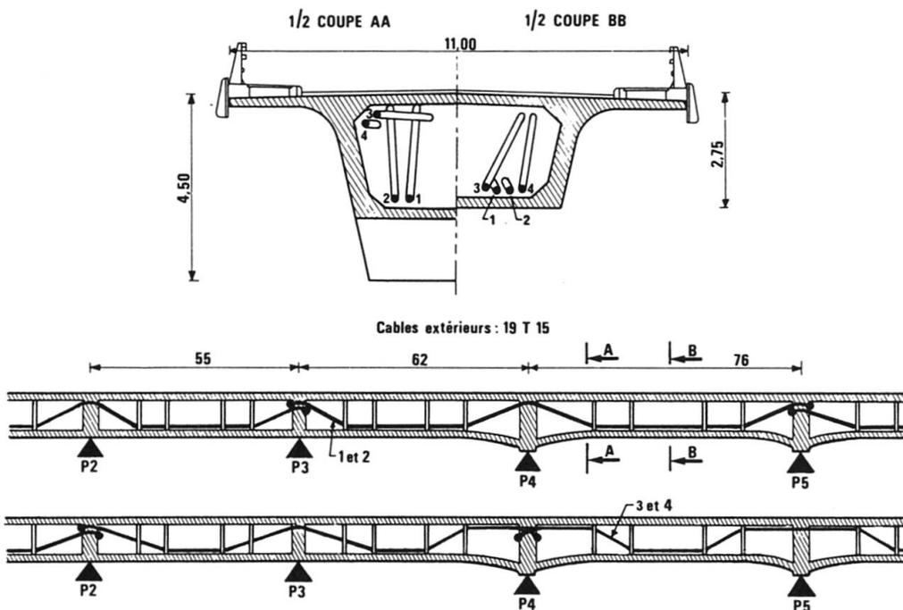
Figure 4 - Cable pattern of Pont-à-Mousson viaduct
