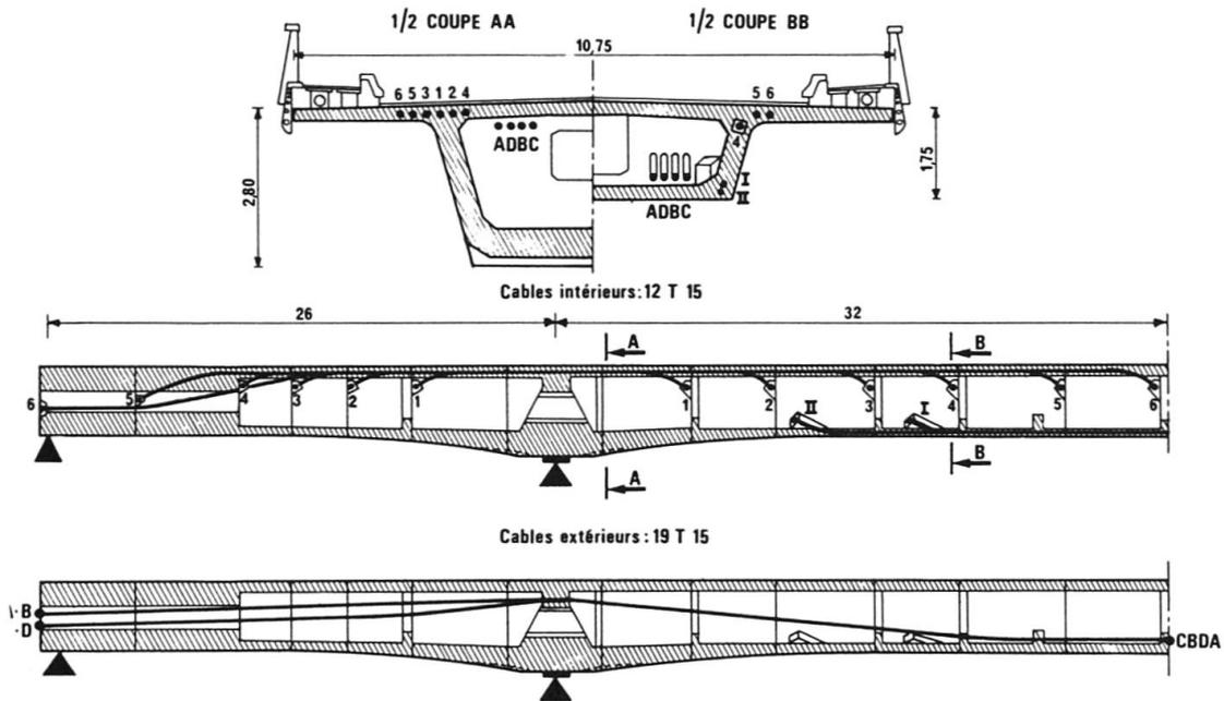
Figure 3 - Cable pattern of La Flèche bridge
