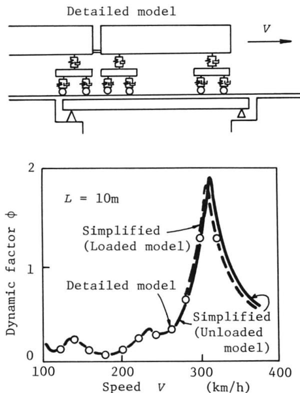
Fig. 3 Effect of wheel base of vehicles and loaded frequency of girder
