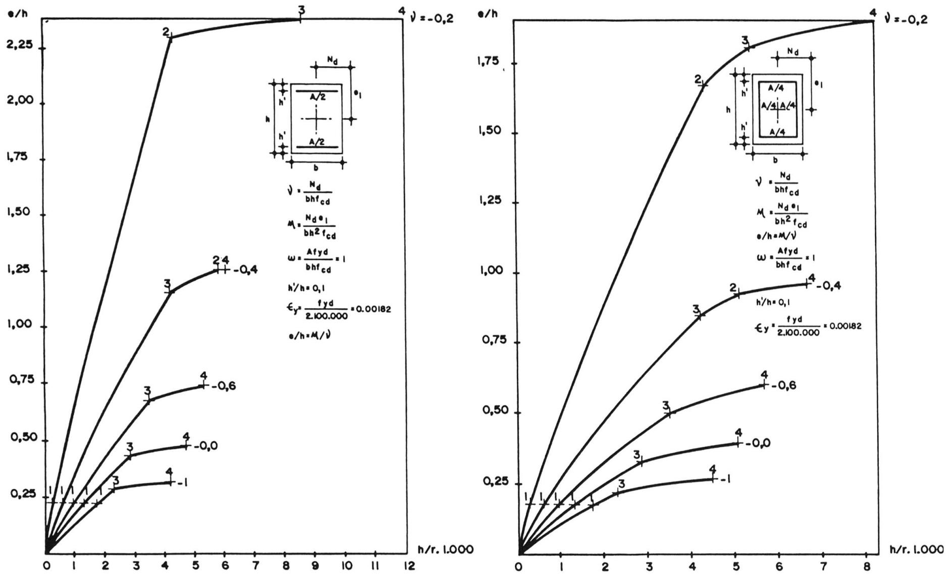
Fig. 3 Characteristic points of the mechanical behaviour curves
