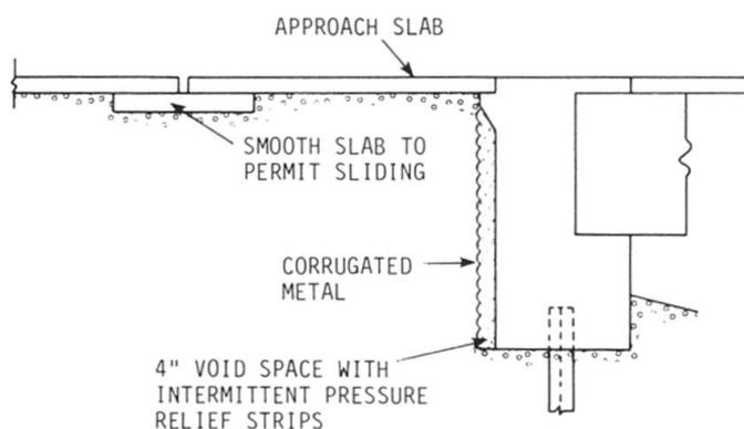
Fig. 6. Integral abutment system with pressure relief strips.
