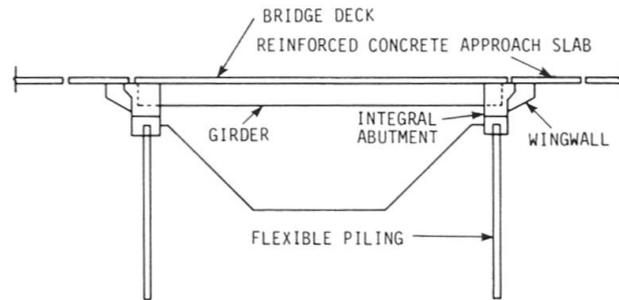
Fig. 3. Cross-section of a bridge with integral abutments.
