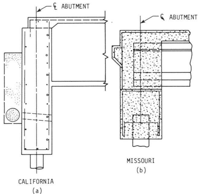
Fig. 4. Integral abutment details.
