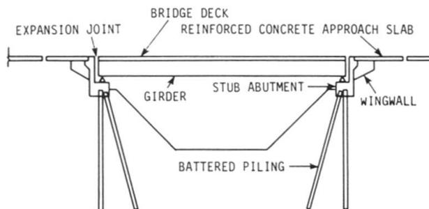
Fig. 1. Cross-section of a bridge with expansion joints.
