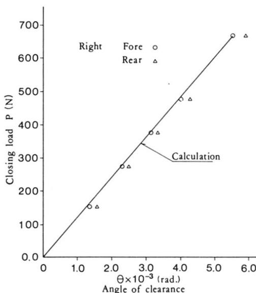
Fig. 20. Closing load of hinge
