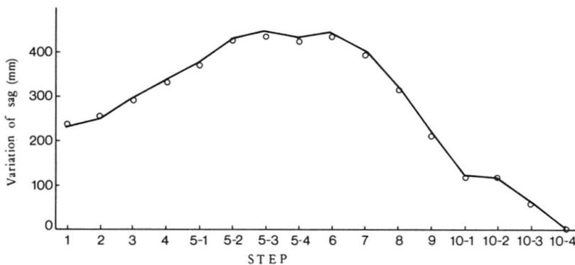
Fig. 10. Variations of sag in center span
