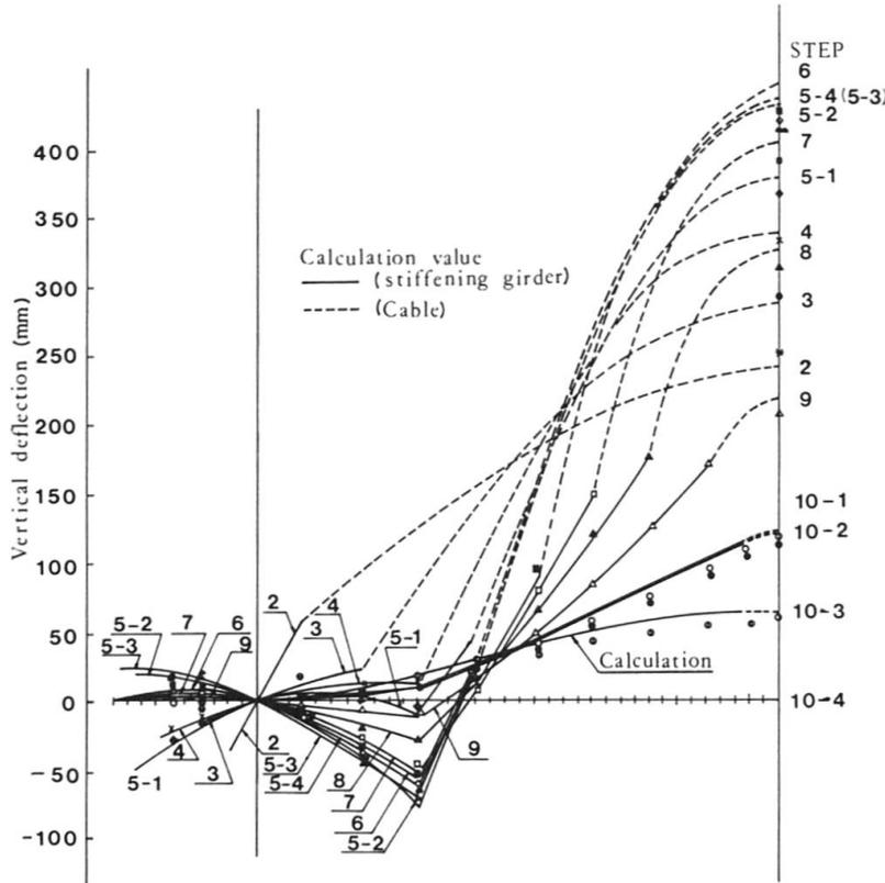
235 mm, showing a difference of 1 %. Deflections of the stiffening girder are shown in Fig. 11. Max. deflection at the tip of the erecting girder in the centerspan is 177 mm on STEP-8, and 59.5 mm on STEP-5-2 at the erection hinge, while the calculated values are 187.2 mm and 63.1 respectively, with a difference of 5 ~ 6 %.
