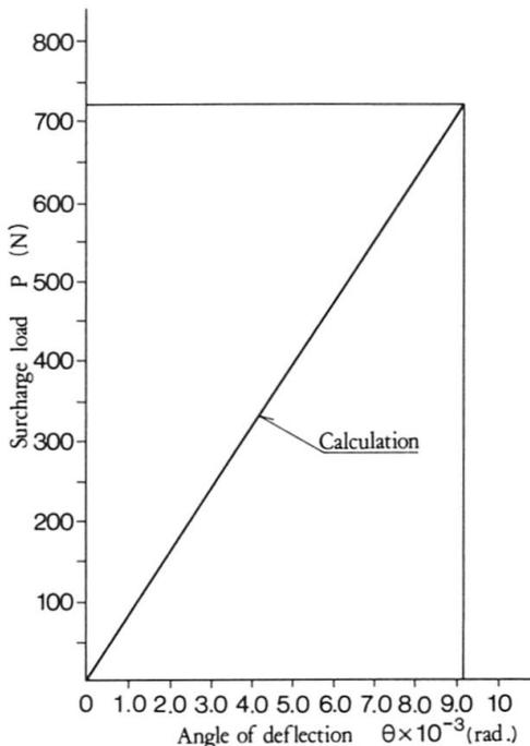
Fig. 22. Surcharge load for closing last block
