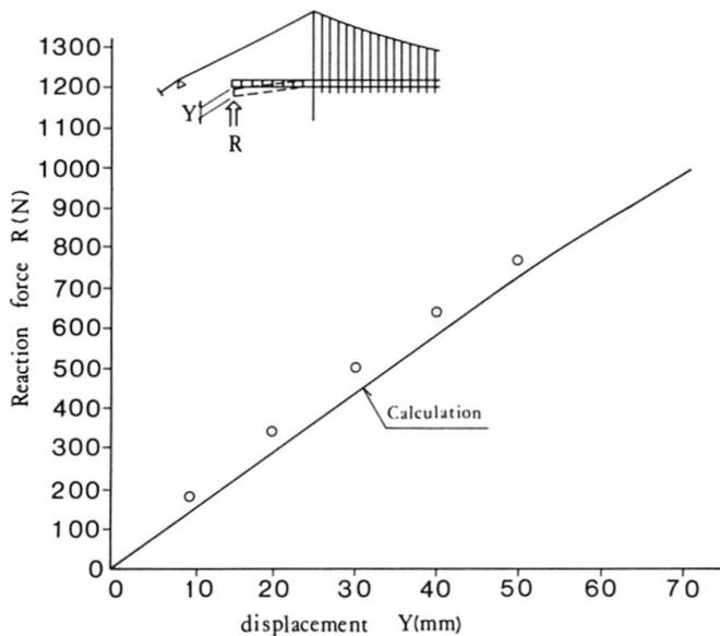
d) Relation between deformation and reaction of the stiffening girder by jack-up loading on the site temporary support in the side span. As shown in Fig. 23, relation between  $Y$  and  $R$  is linear, therefore on STEP-5-1, where  $R/Y \approx 14.7 \text{ N/mm}$ ,  $Y = 72 \text{ mm}$  would be required, and where  $R = 14.7 \times 72 = 1,058.4 \text{ N}$  in the model, which means  $Y = 1.8 \text{ m}$ ,  $R = 10,780 \text{ kN/bridge}$  in the prototype.
