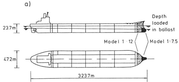
Fig.6 Collision tests of the GKSS with 195,000 dwt tanker "Esso Malaysia"
