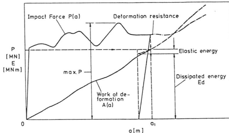
Minorsky has systematically investigated collisions between ships for the design of the American nuclear powered ship N/S "Savannah", [11]. The finding of that study was that a linear correlation exists between the volume of the ship's steel deformed in the collision of both ships and the absorbed energy, Figure 2.
