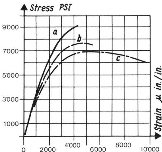
Fig. 2 Compressive stress strain curves for polymer-concrete. Curve a, MMA; curve b, 95 wt % MMA - 5 wt % BA, curve c, 80 wt % MMA - 20 wt % BA.
