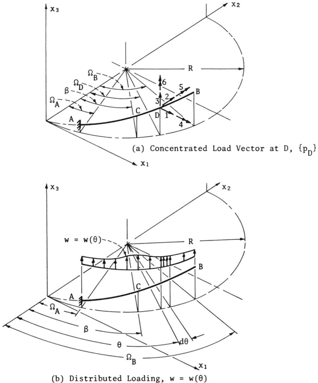
FIG. 2 CONCENTRATED AND DISTRIBUTED LOADINGS ON HELICOIDAL MEMBER AB.
