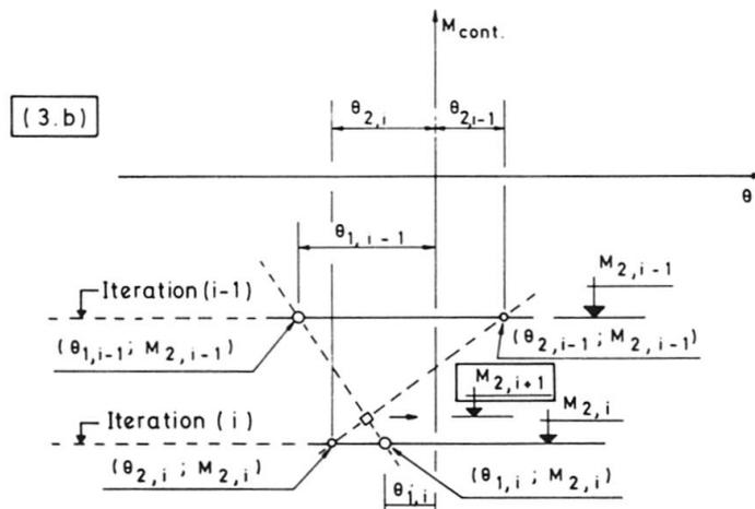
FIGURE 3.- Iteration procedure for continuity bending moment determination
