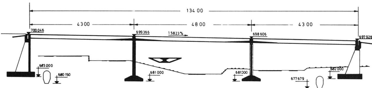
FIGURE 4. - "Cuzco - Barajas" Bridge over motorway M-30 in Madrid (Spain). Longitudinal section.
