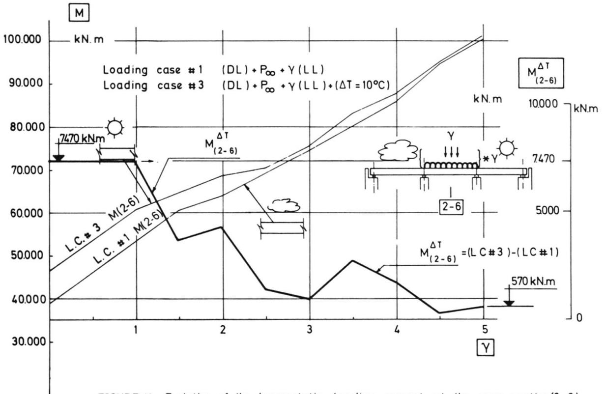
FIGURE 11.- Evolution of the hyperstatic bending moment at the cross-section (2-6) due to a temperature gradient,  $\Delta T = 10^\circ C$
