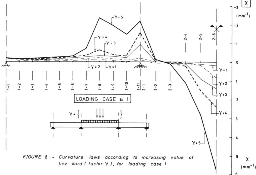
FIGURE 8.- Curvature laws according to increasing value of live load (factor  $\gamma$ ), for loading case 1
