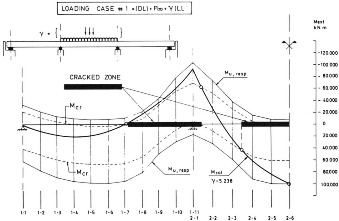
FIGURE 7.- Final state of the continuous deck at collapse, for loading case 1
