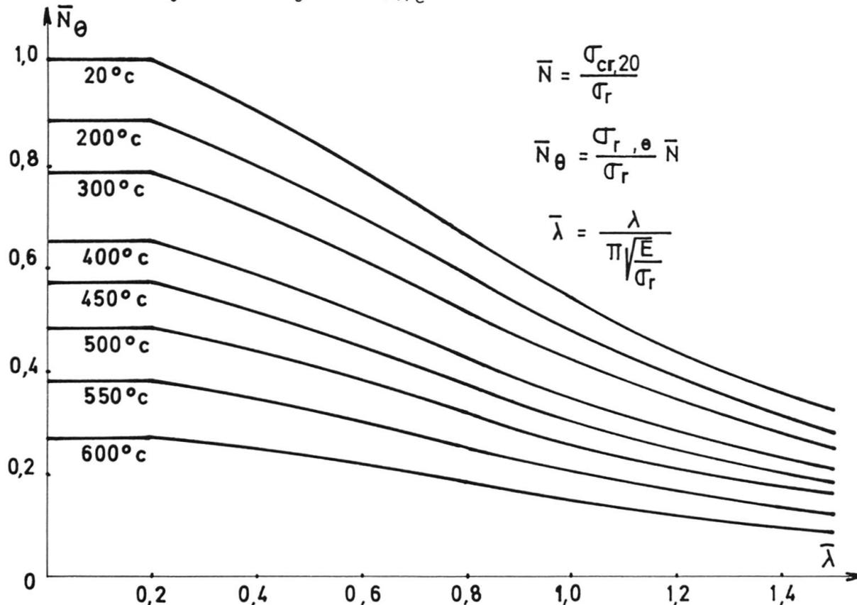
Fig. 2. Non dimensional buckling curves at elevated temperature.
