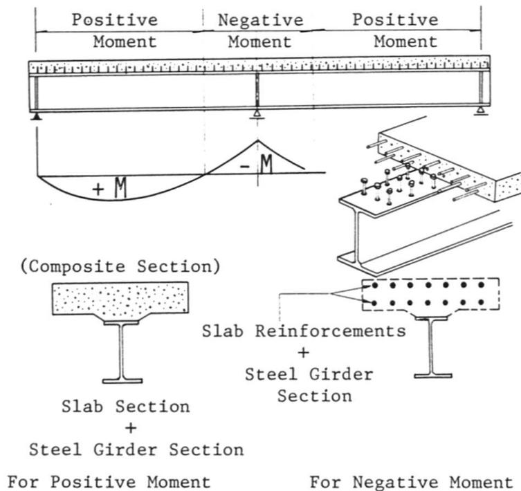
Fig.6 Design Model of Non-Prestressed Continuous Composite Girder
