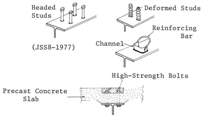
Fig. 1 Shear Connectors
