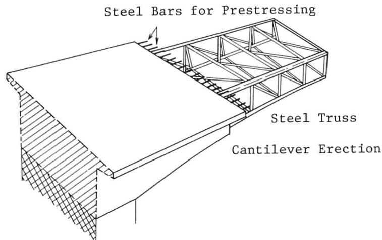
Fig. 11 Steel Prestressed Concrete Erection Method (SPC Method)
