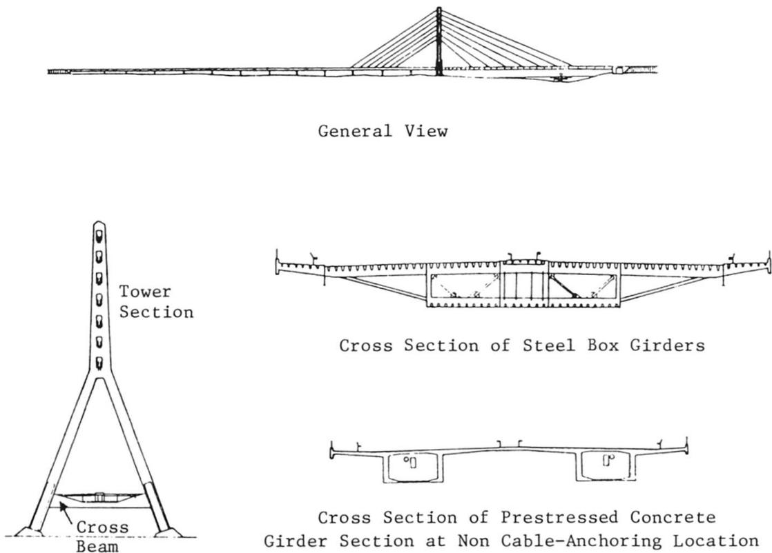
Fig.16 General View and Cross Section of Flehe Bridge
