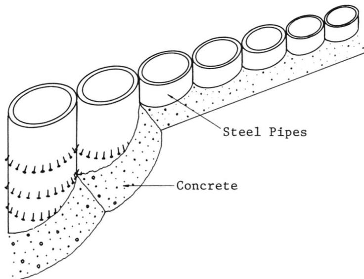
Fig. 15 Composite Continuous Underground Wall
