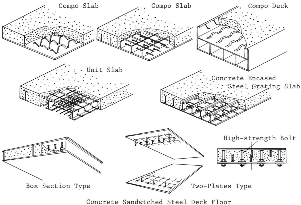
Fig. 8 Composite Slabs and Deck Floor
