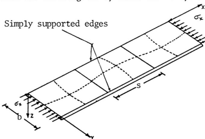
FIG. 2: Simply supported plate with axial loading
