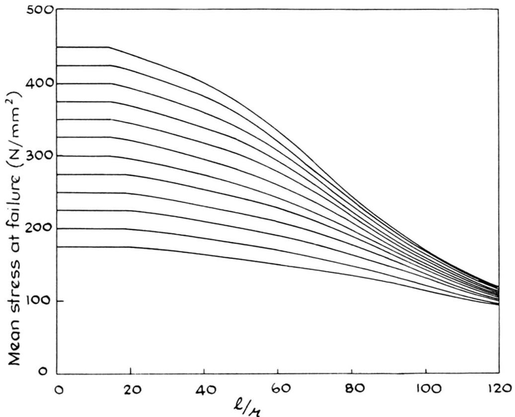
FIG. 6 : Slenderness Ratio vs. mean stress at failure
