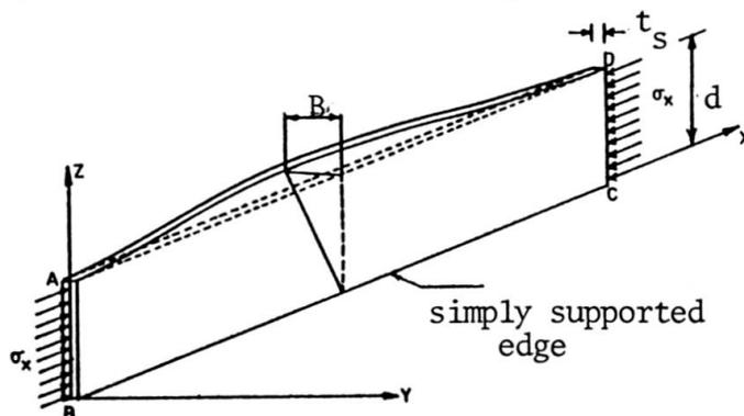
FIG.4: Axially loaded plate with one edge free to wave
