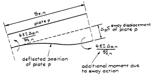
Fig. 5 Sway displacement of a typical plate
