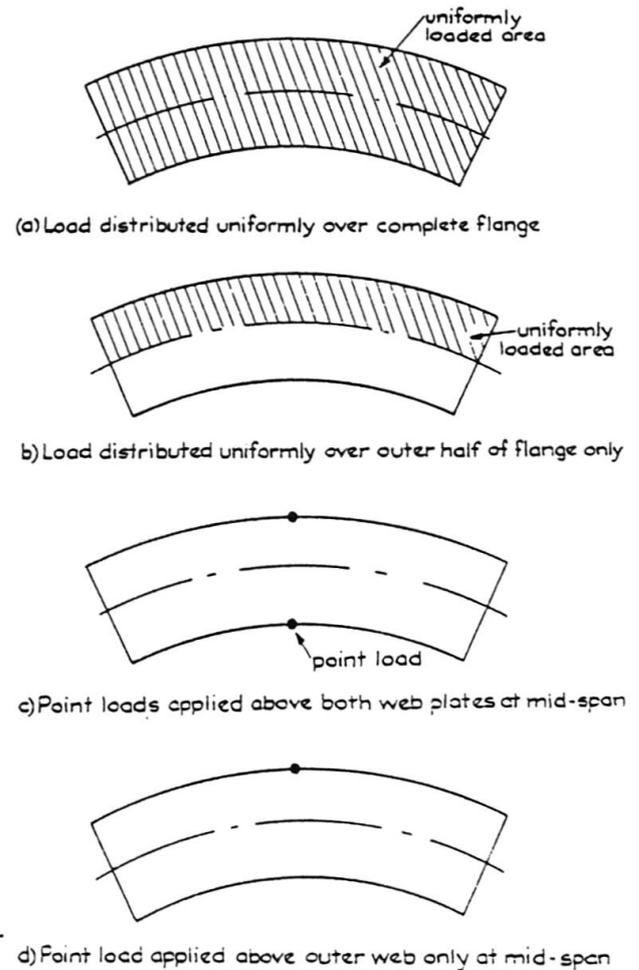
Fig. 10 Details of loading conditions considered
