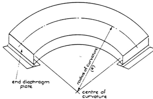
Fig. 1 Typical curved box girder considered in the analysis
