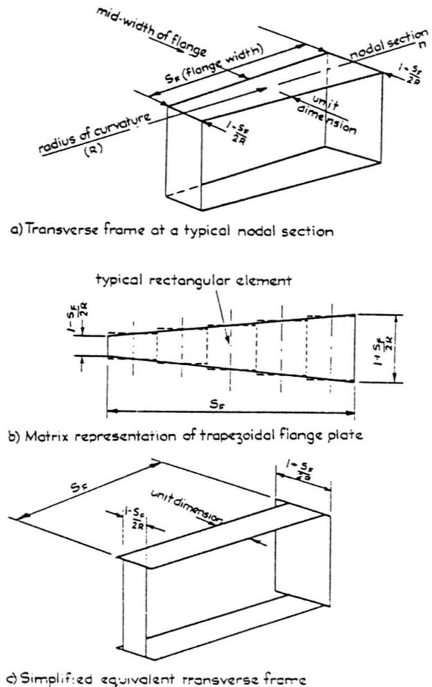
Fig. 3 Details of the transverse frame analysis
