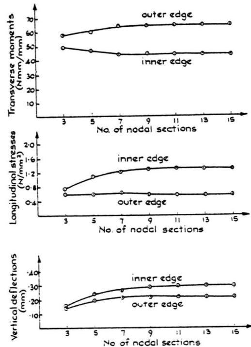
Fig. 6 Convergence of nodal section solution for a typical sand/araldite box
