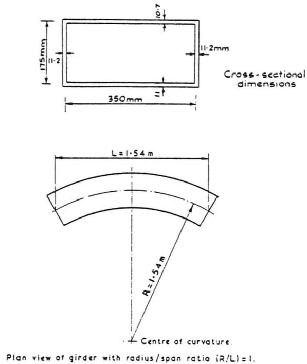
Plan view of girder with radius/span ratio  $(R/L) = 1$ .
