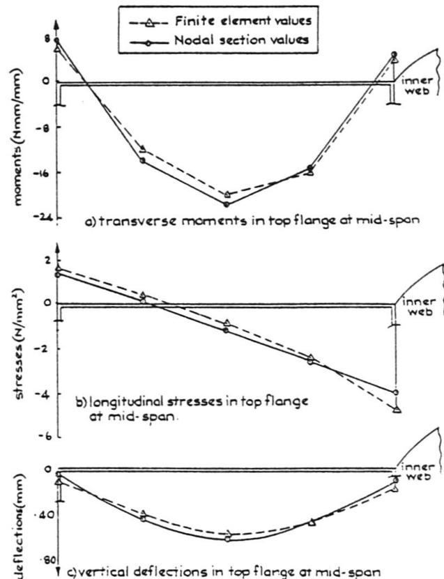
Fig. 16 Comparison of values for steel girders
