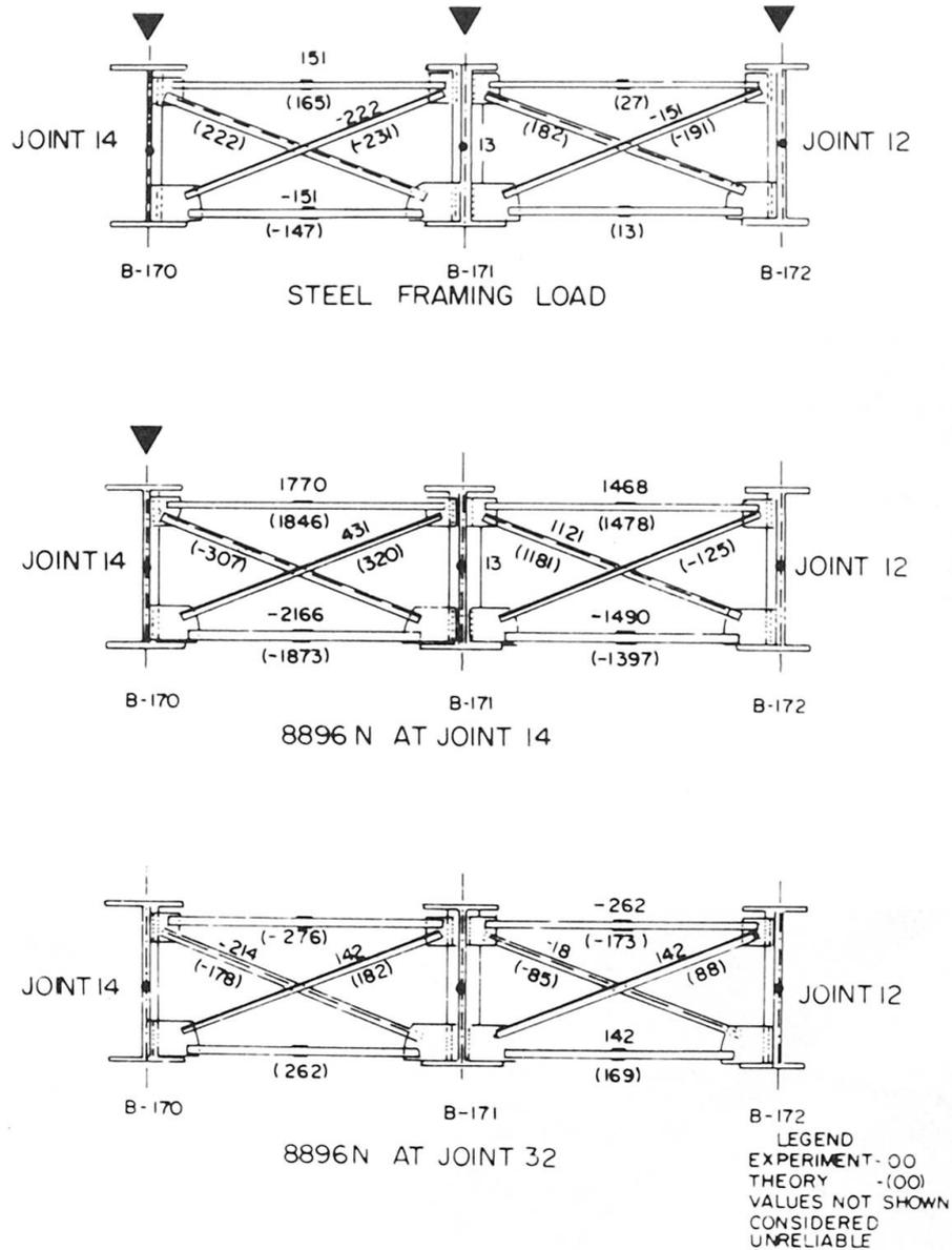
Fig. 13 Analytical and Experimental Forces in Diaphragm Members
