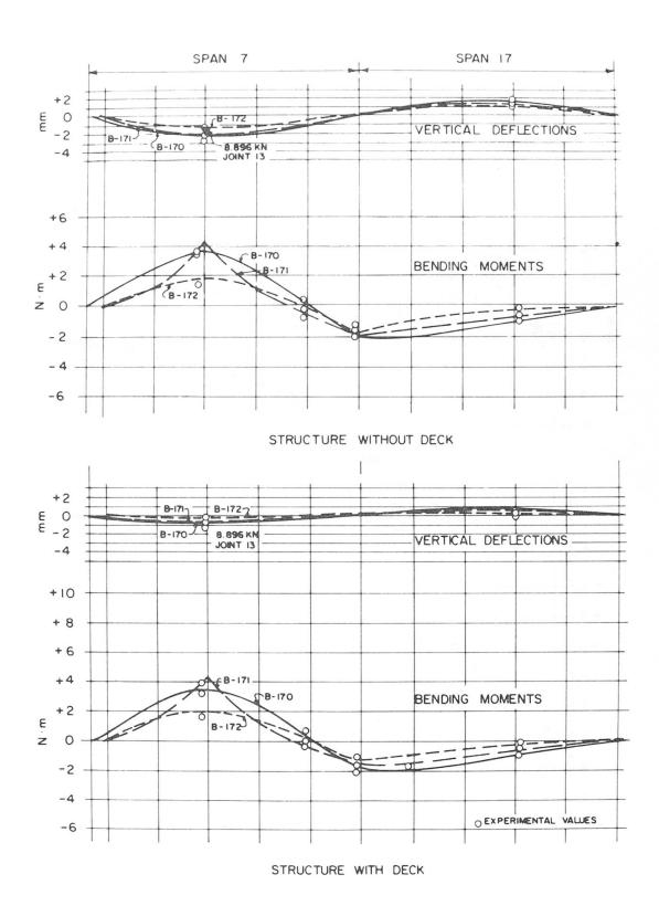
Fig. 10 Analytical and Experimental Moments and Deflections for Load at Joing 13 Small Scale Structure without Deck and with Deck
