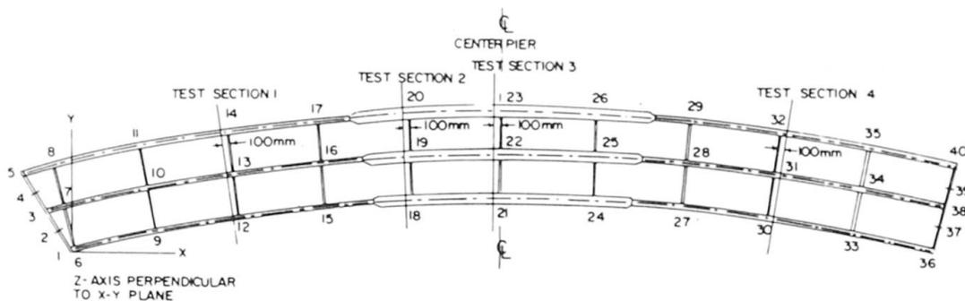
Fig. 7 General Coordinate System and Test Section Locations
