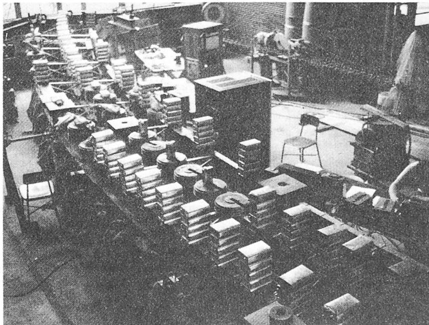
Fig. 3 Dead Loading on Small Scale Seekonk River Bridge
