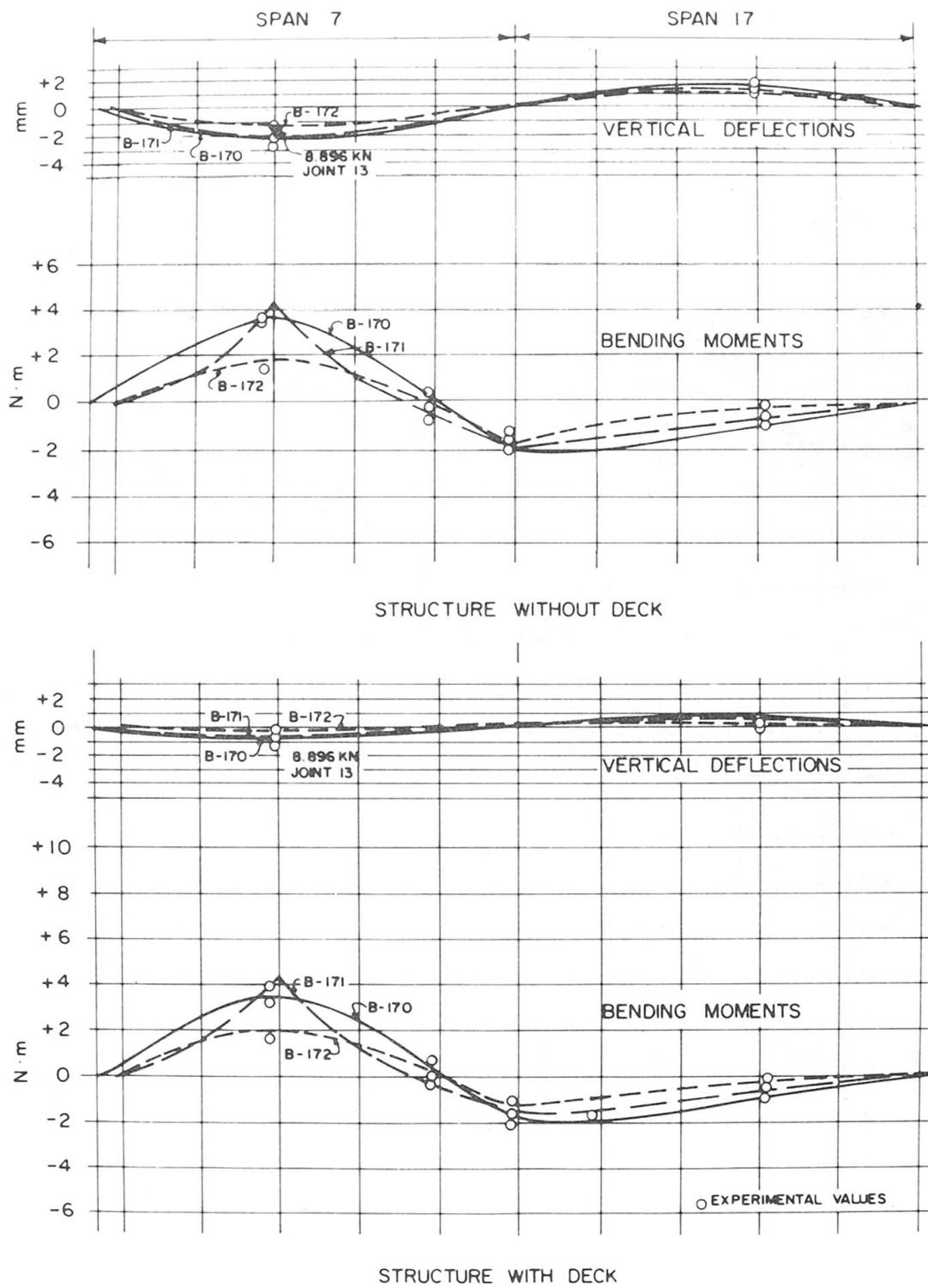
Fig. 10 Analytical and Experimental Moments and Deflections for Load at Joing 13 Small Scale Structure without Deck and with Deck
