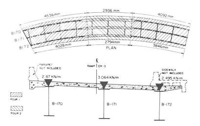
Fig. 5 Wet Concrete Loading Sequence as Poured on Prototpye Structure
