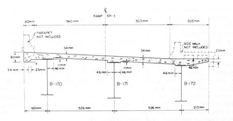
Fig. 2 Section Through Small Scale Bridge
