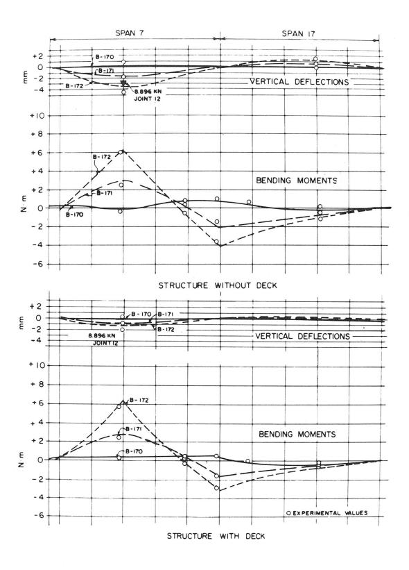
Fig. 9 Analytical and Experimental Moments and Deflections for Load at Joint 12 Small Scale Structure without Deck and with Deck
