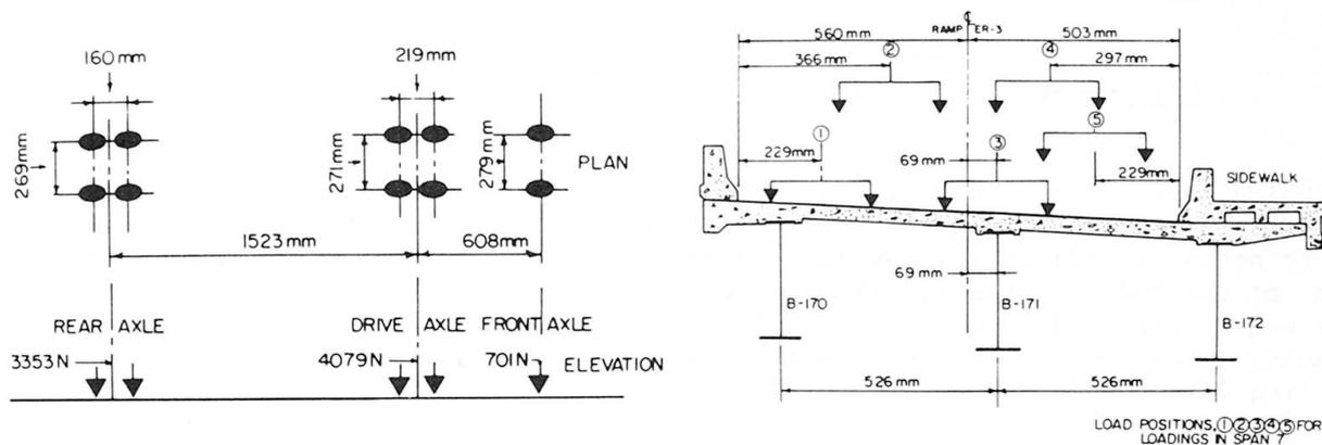
Static Live Load Forces and Dimensions Transverse Locations of Live Loads
