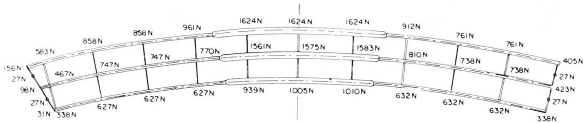
Fig. 4 Steel Framing Loads Transferred to Mathematical Joints
