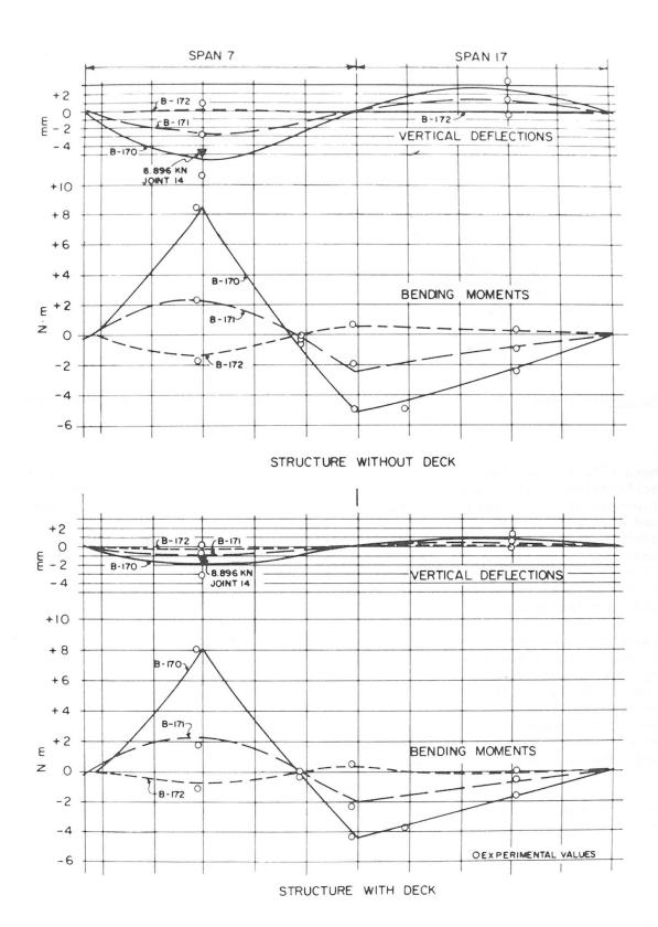
Fig. 11 Analytical and Experimental Moments and Deflections for Load at Joint 14 Small Scale Structure without Deck and with Deck
