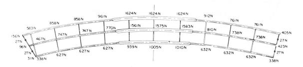
Fig. 4 Steel Framing Loads Transfered to Mathematical Joints
