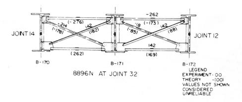
Fig. 13 Analytical and Experimental Forces in Diaphragm Members
