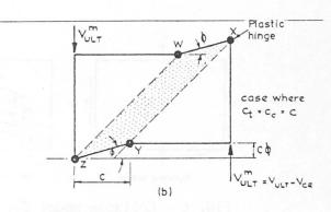
FIG. 7 - Collapse mode for pure shear
