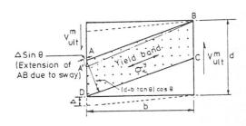
$\frac{\text{FIG. 8}}{\text{c}}$  - Yield band when c = 0 (true Basler solution).
