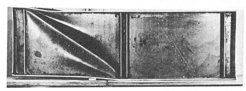
FIG. 4 - View of a failed girder showing failure sway mechanism
