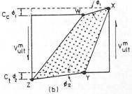
FIG. 15 - Collapse mechanism developed in a panel loaded in shear and bending.
