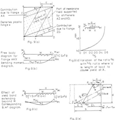
FIG. 9 - Stress conditions in a shear web due to the membrane field.
