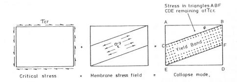
FIG. 2 - Ultimate load mechanism developed by Basler et al [4,5]
