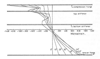
FIG. 12 - Mid plate strains developed in girder TG5-2 when subjected to a bending moment [24].
