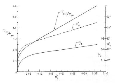
FIG. 11 - Relationship between  $\tau_{ult}/\tau_{yw}$ ,  $\Theta_m$ , c/b and  $M_p^*$  for panel with an aspect ratio of 2 and d/t ratio of 200:1.
