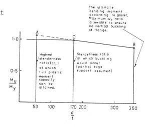
FIG. 14 - Relationship between the ratio  $M_{1}/M_{y}$  and the d/t ratio as proposed by Basler and Thurlimann [25]  $(\sigma_{y}$  = 30000 psi).
