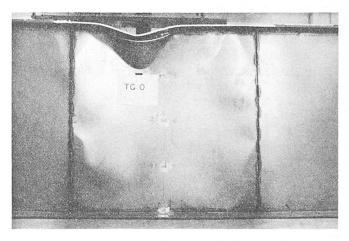
FIG. 13 - Illustration of failure due to inward collapse of compression flange [24].
