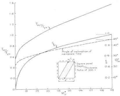
FIG. 10 - Relationship between  $\tau_{\rm ult}/\tau_{\rm yw}$ ,  $\theta_{\rm m}$ , c/b and M<sup>\*</sup><sub>p</sub> for panel of aspect ratio 1 and d/t ratio 200:1. Vertical stiffeners assumed to remain straight.
