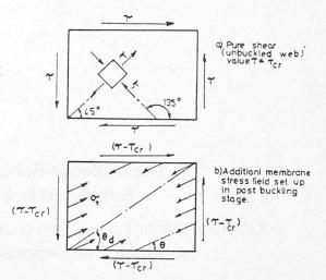
FIG. 1 - Stresses in a panel subjected to shear
