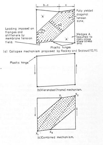
FIG. 3 - Mechanisms involved in collapse of shear panel.
