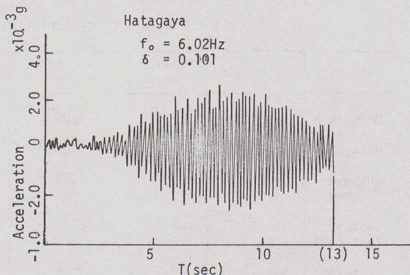
Fig. 4 Actual response at 1/2 of the span
