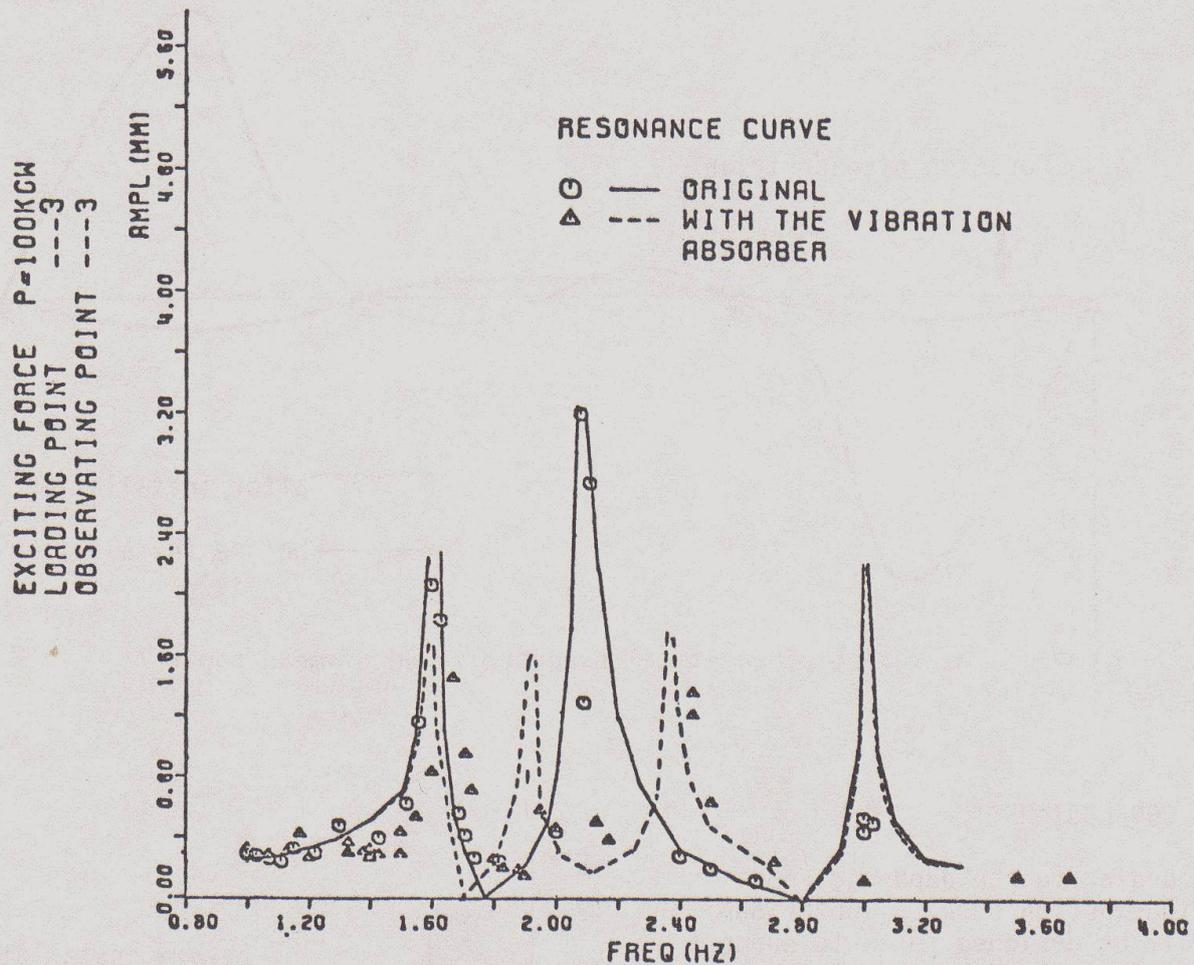
Fig. 14 Resonance curve before and after installation
