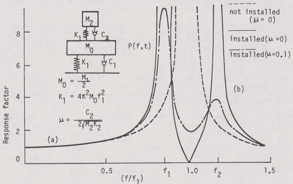
Fig. 11 Resonance curve
