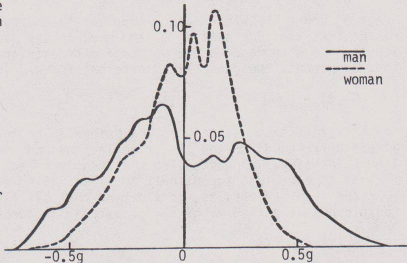
Fig. 3 Probability density function for acceleration of pedestrians
