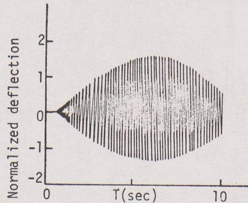
Fig. 7 Simulation of response at Hatagaya Footbridge
