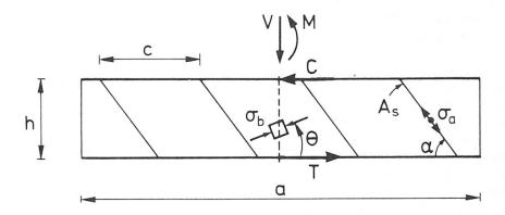
Fig. 2 Truss model of reinforced concrete beam
