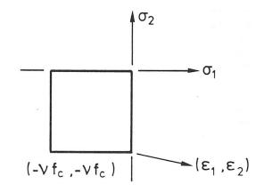
Fig. 3 Yield locus for concrete in plane stress
