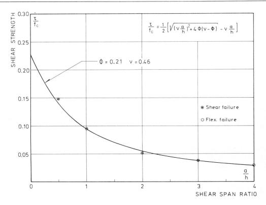
Fig. 10 Shear tests on beams without web reinforcement (ROIKJAER [29])
