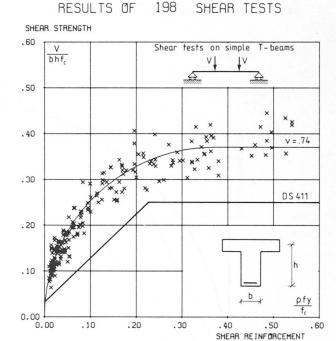
Fig. 8 Shear test results compared with web crushing criterion and Danish Code
