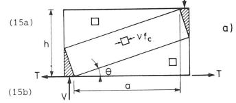
Fig. 9 Shear failure of beams without web reinforcement
