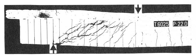
Fig. 5 Shear failure of beam with web reinforcement (BRÆSTRUP et al [2])
