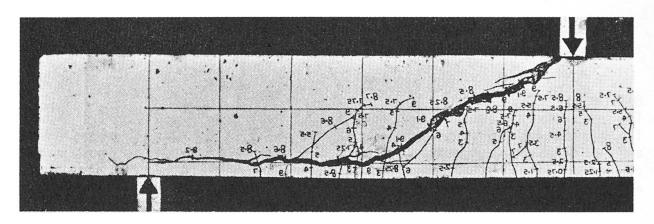
Fig. 1 Diagonal tension failure of beam without web reinforcement (reproduced from TAYLOR [32])
