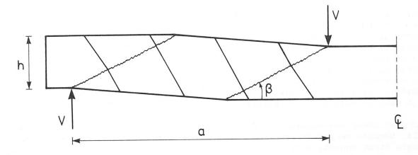
Fig. 4 Shear failure mechanism for reinforced concrete beam
