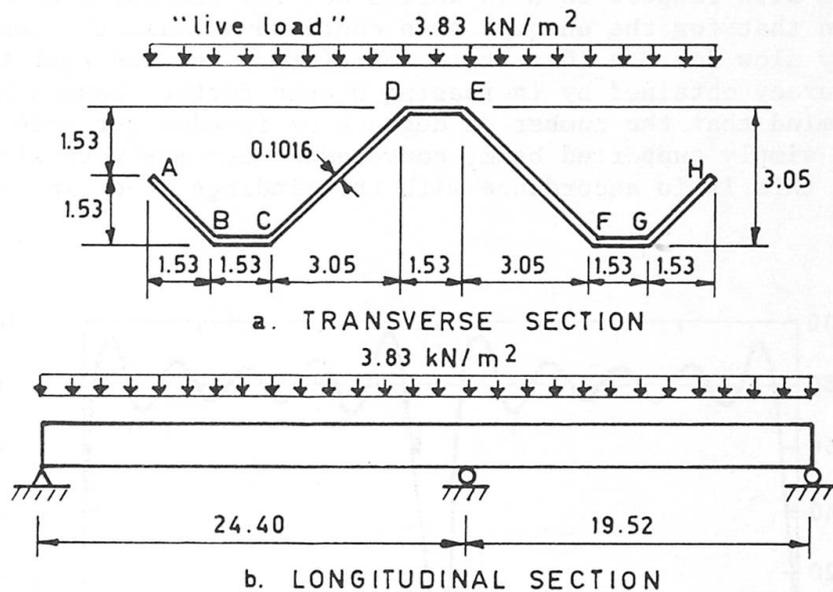
Fig.3 Dimensions (in m) and loading for Example 1
