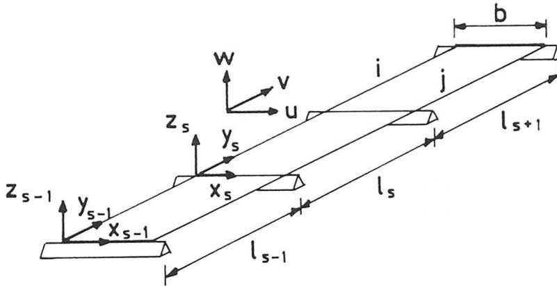
Fig. 1 A Typical continuous finite strip
