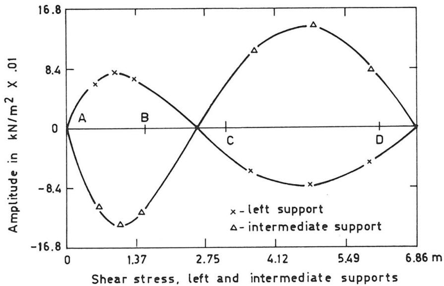
Fig.5 Example 1. Transverse distribution of shear stress
