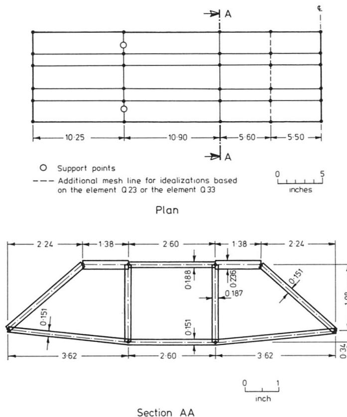
Fig.5 Straight three cell box girder bridge model.
