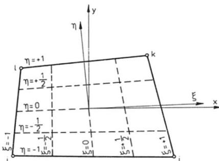
Fig.2 Quadrilateral element and generalized co-ordinate system
