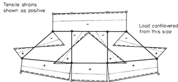
(a) Distribution of longitudinal outer surface strains
