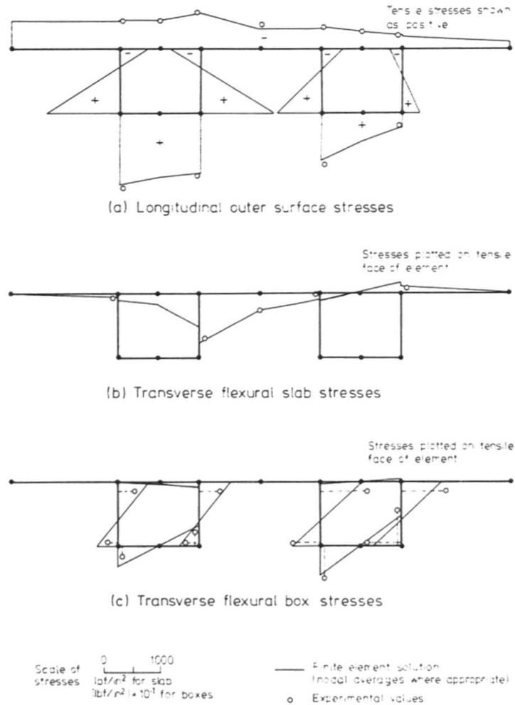
Fig 12 Composite twin cell box girder bridge model
