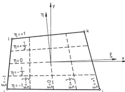
Fig.2 Quadrilateral element and generalized co-ordinate system
