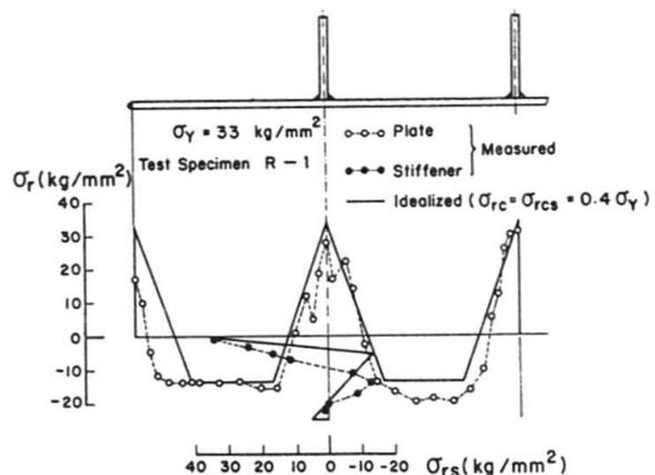
Fig. 11 Measured and Idealized Residual Stress Patterns
